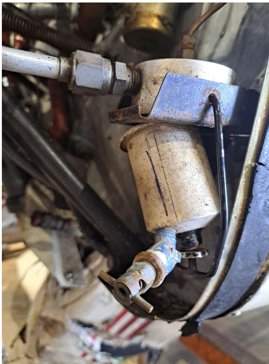
Photograph 7 - Gascolator Assembly (Piper Photo)
