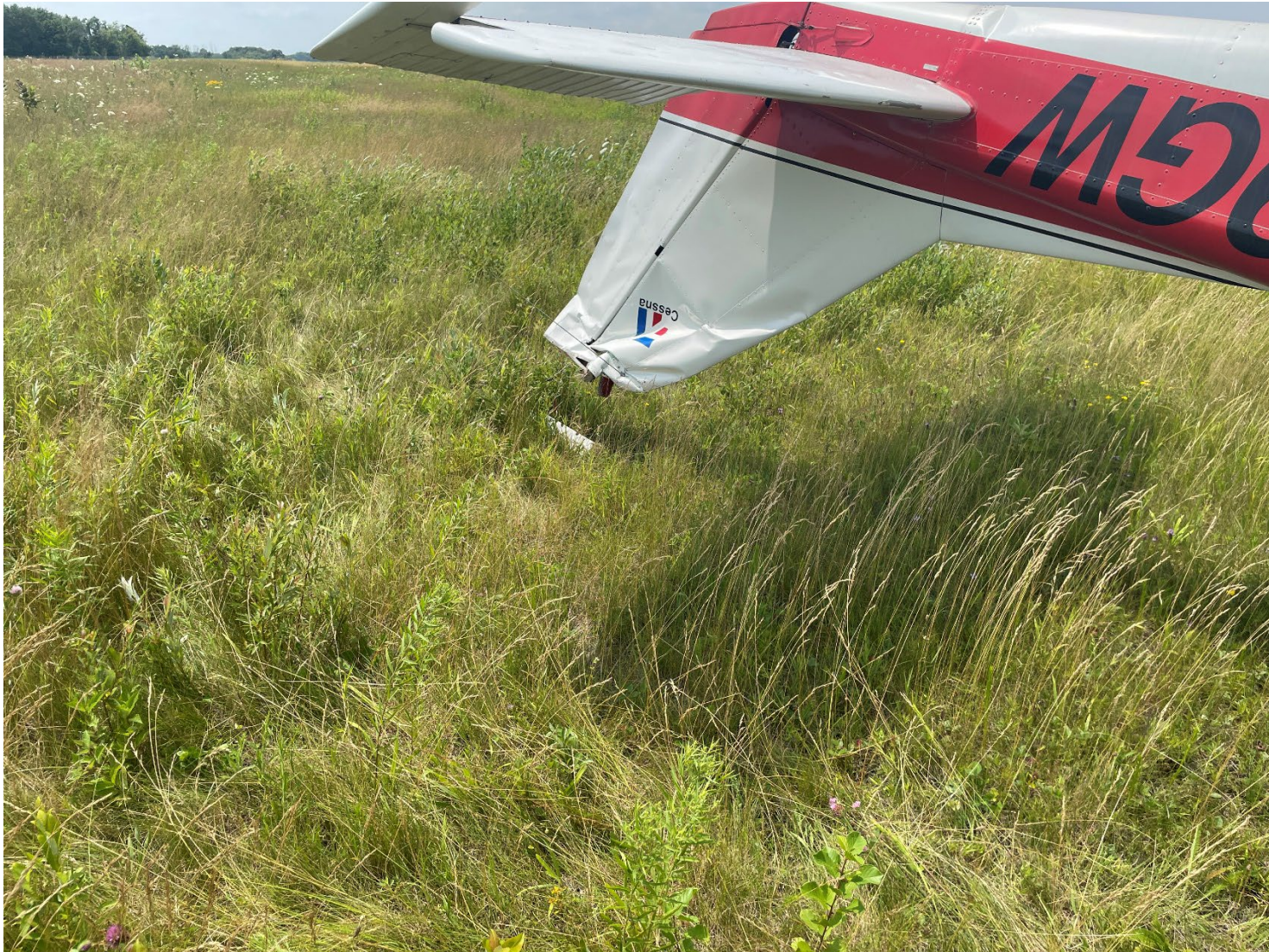
Photograph 3 - Vertical Stabilizer Damage (Courtesy of FAA)
