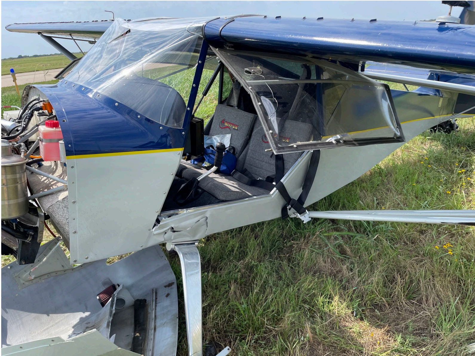
Photograph 2 - Lower Fuselage Damage (Courtesy of Highway Patrol)
