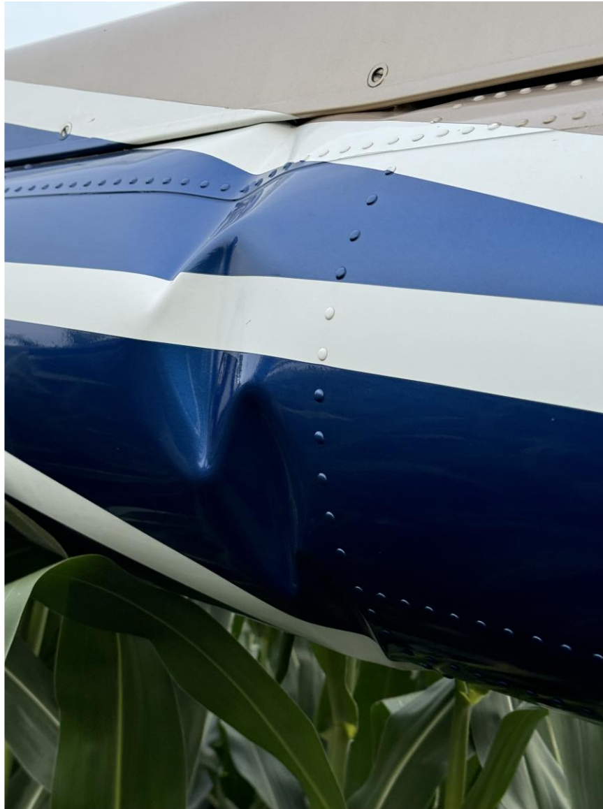
Photo 6 - Tailboom damage (Courtesy of Pilot)
