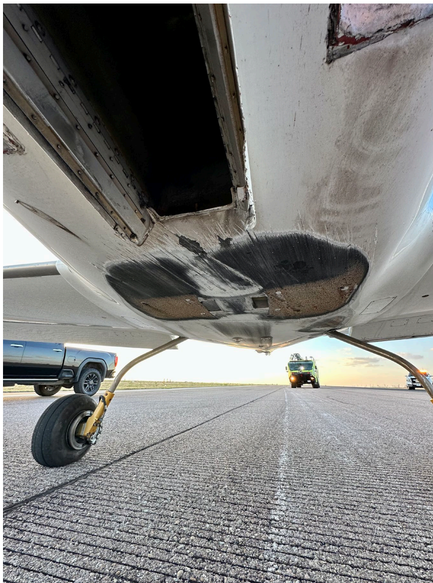
Photograph 2 - View of bottom of fuselage showing exposed core material (Courtesy of FAA)
