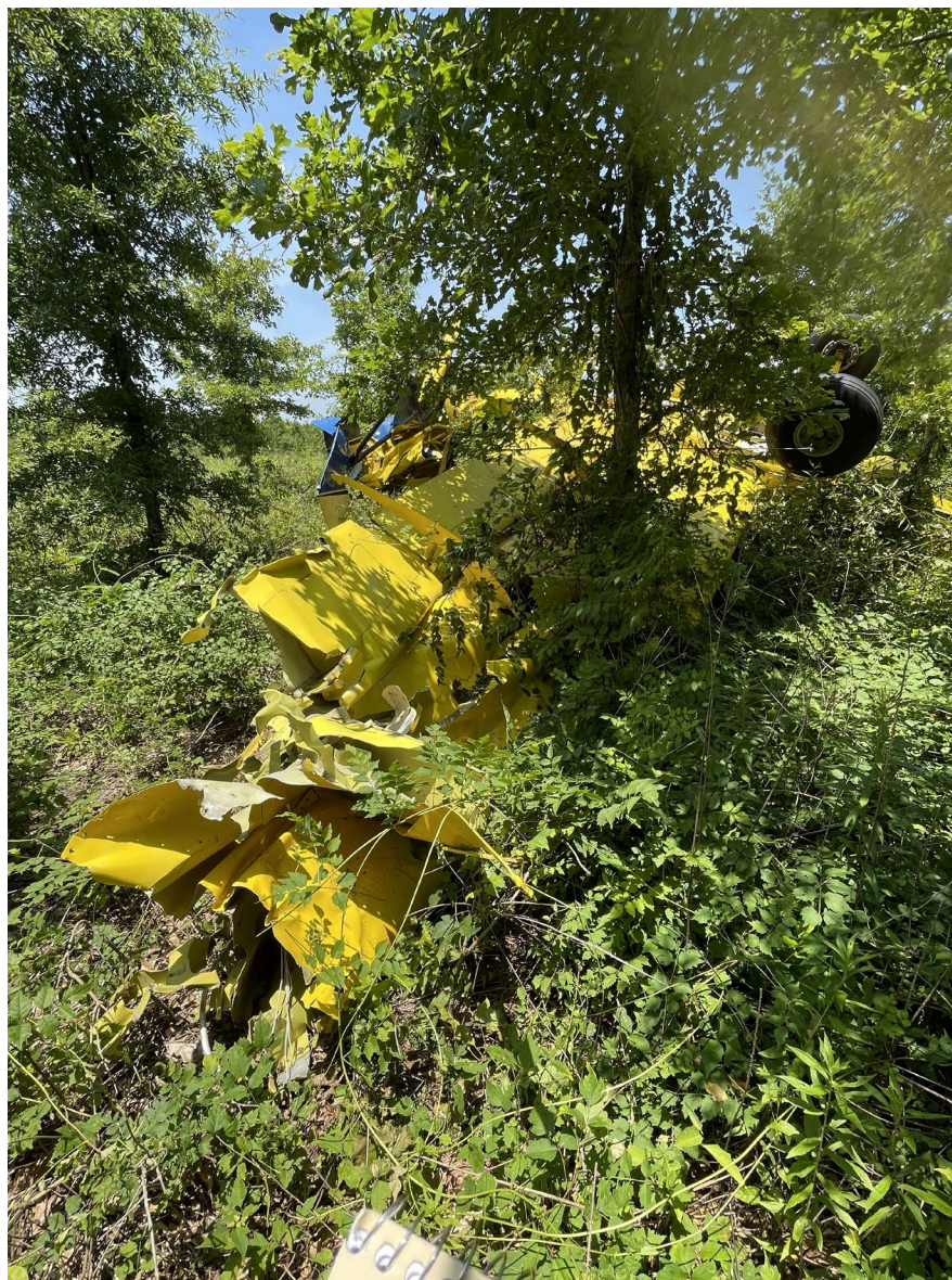
Photograph 2 - Left Wing Substantial Damage (Courtesy of FAA)
