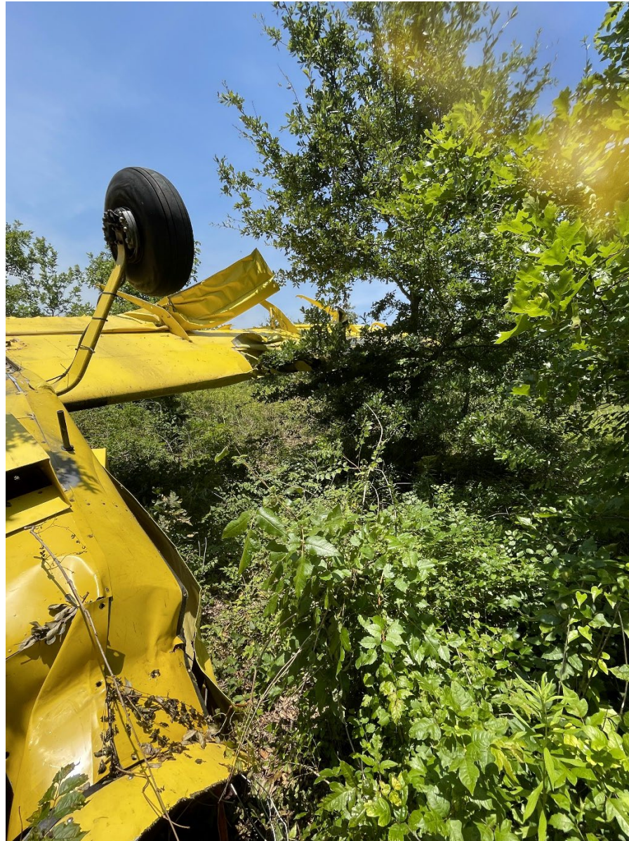
Photograph 3 - Fuselage & Right Wing Substantial Damage (Courtesy of FAA)
