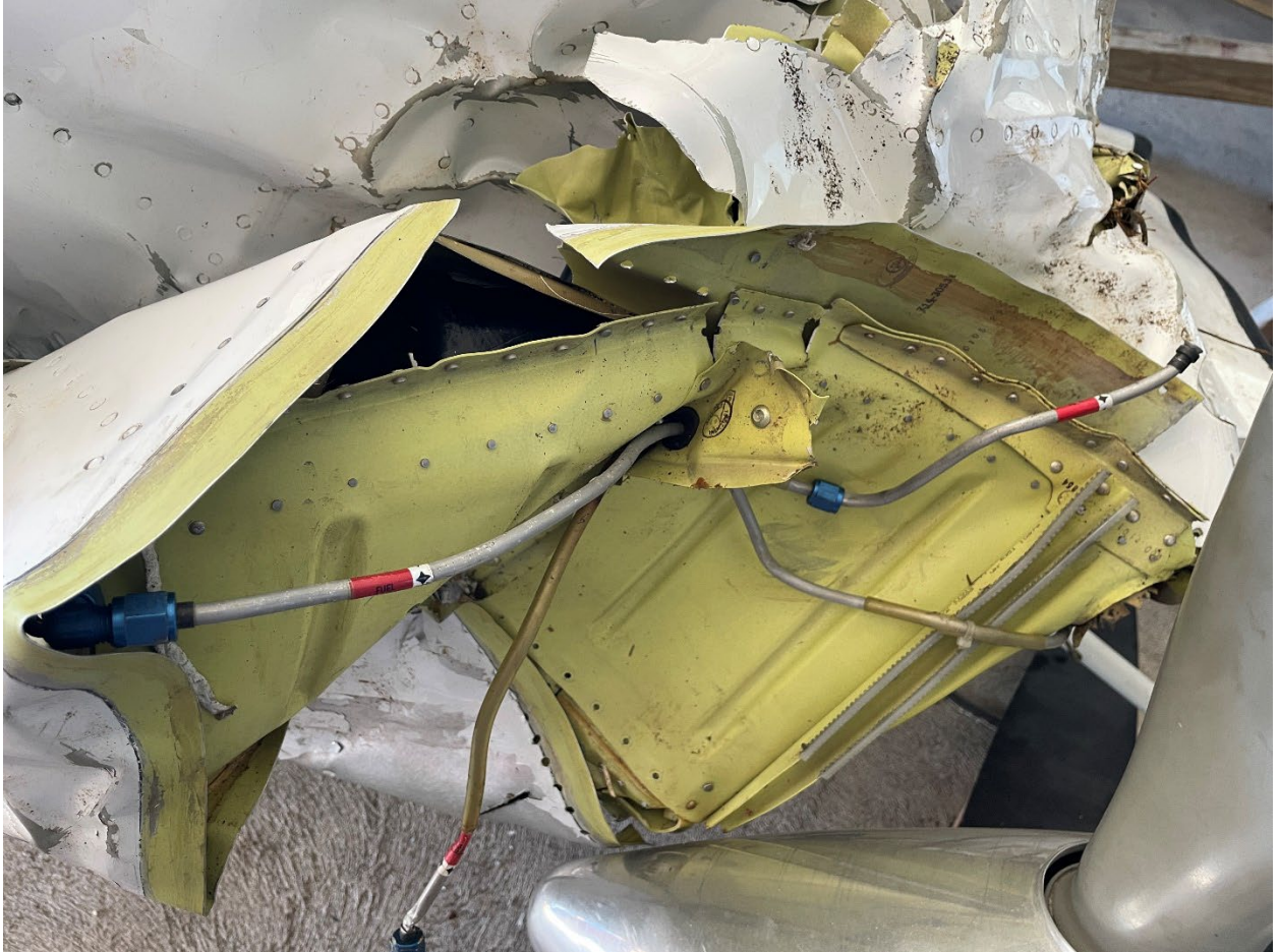
Figure 3. Damaged Left wing fuel supply and vent line.
