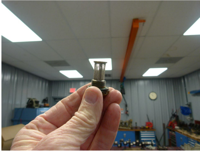
Picture 8 Fuel Control Screen
