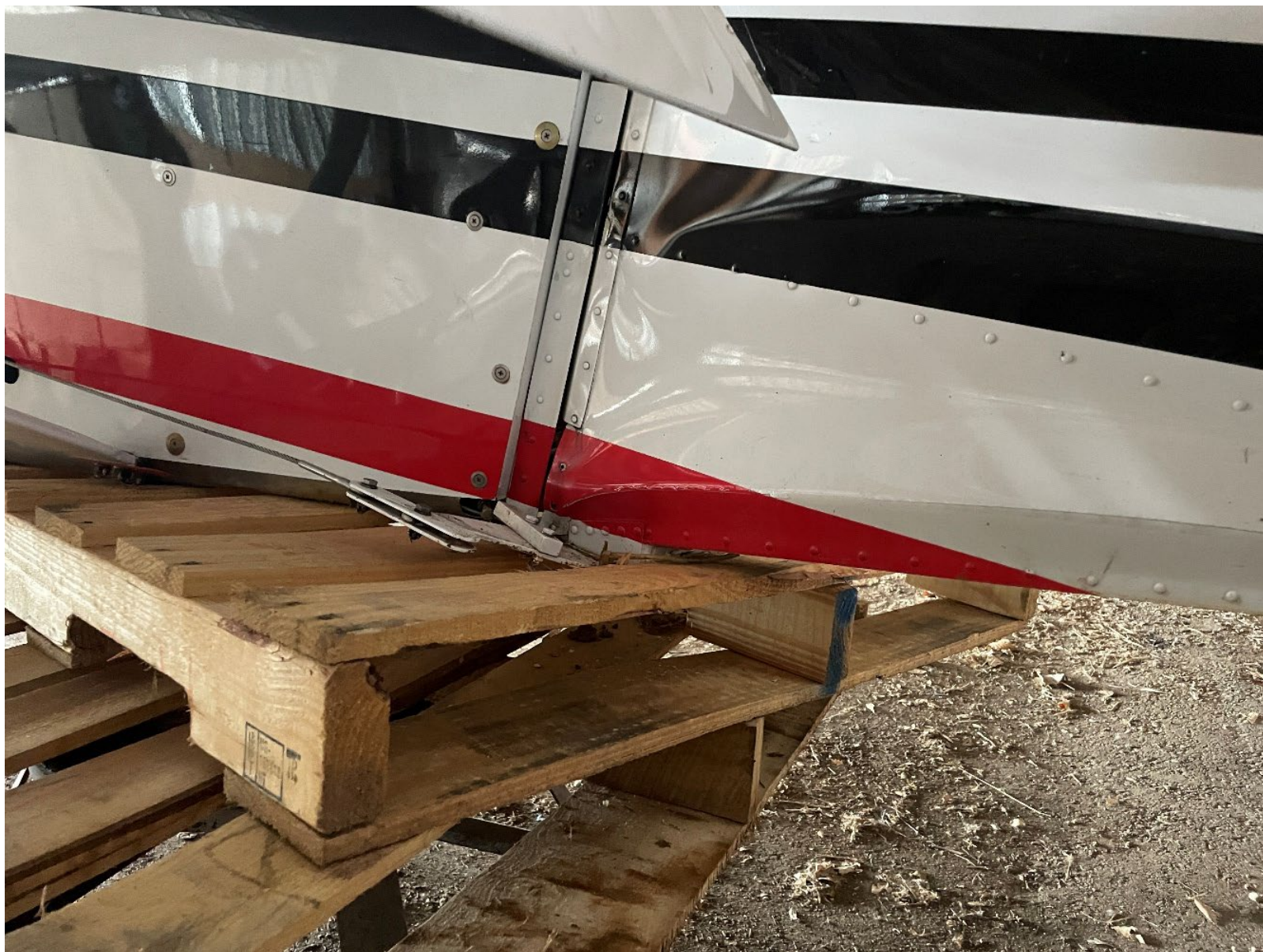
Photograph 6 - View of the substantial damage sustained to the rudder
