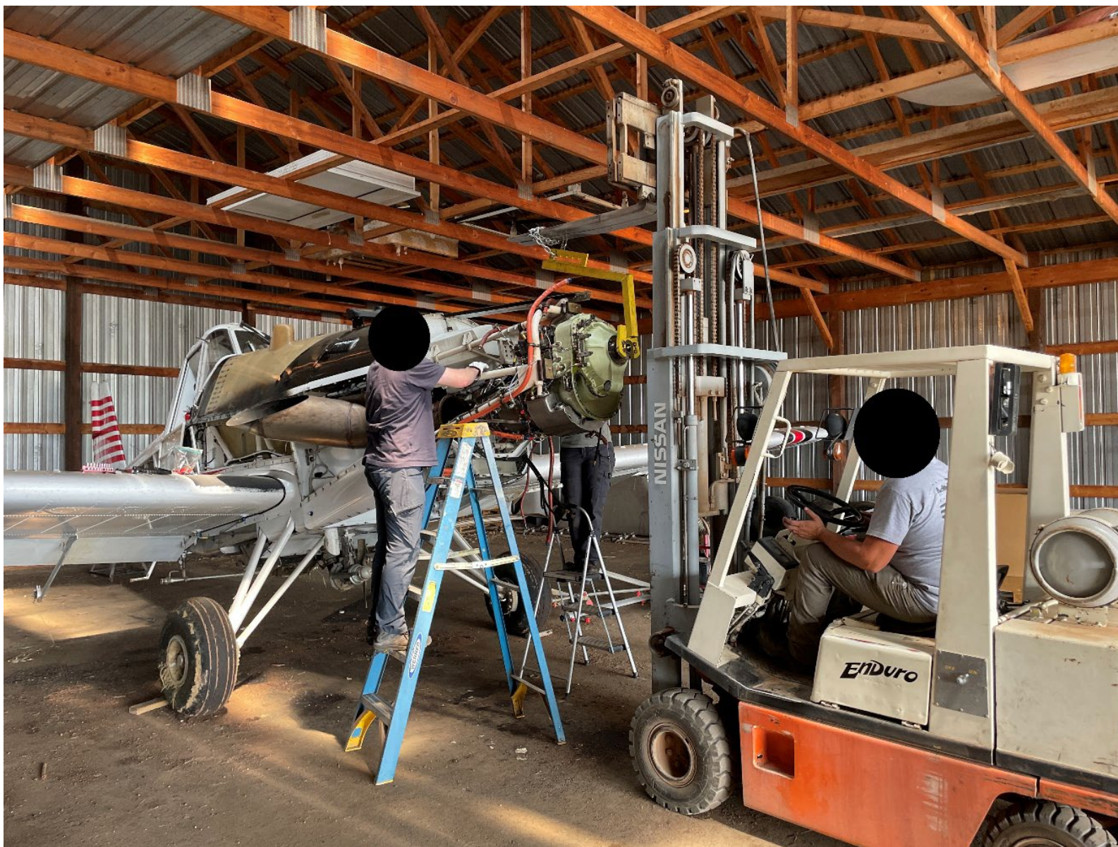
Photograph 7 - View of the engine being removed from the airframe
