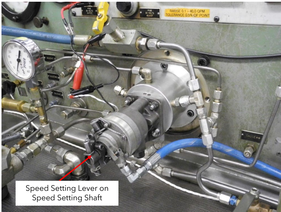
Figure 15. PG Mounted onto Test Stand
