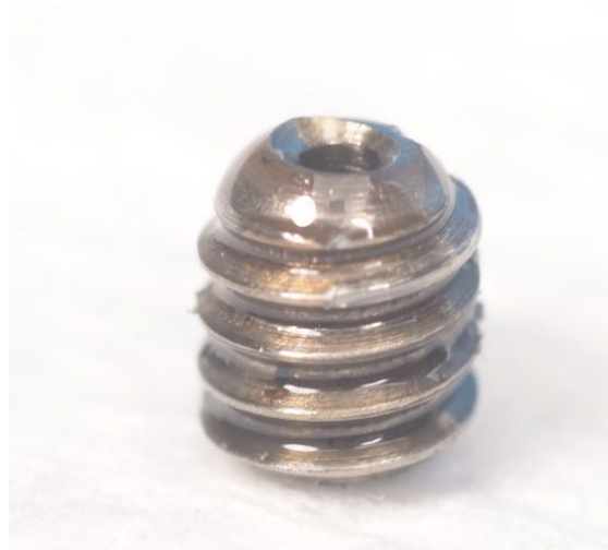
Figure 25. PG Reset Orifice - Clean
