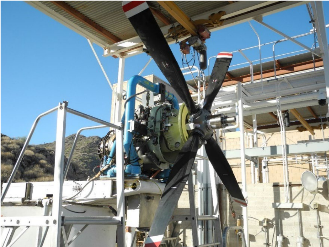
Figure 10. TPE331 Event Engine in Propeller Stand
