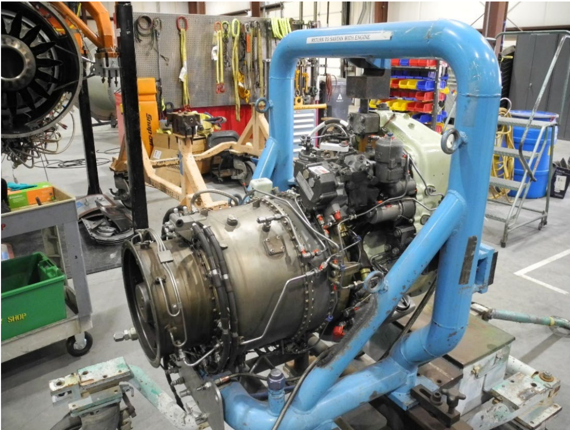
Figure 3. Engine Placed into the Propeller Stand Collar
