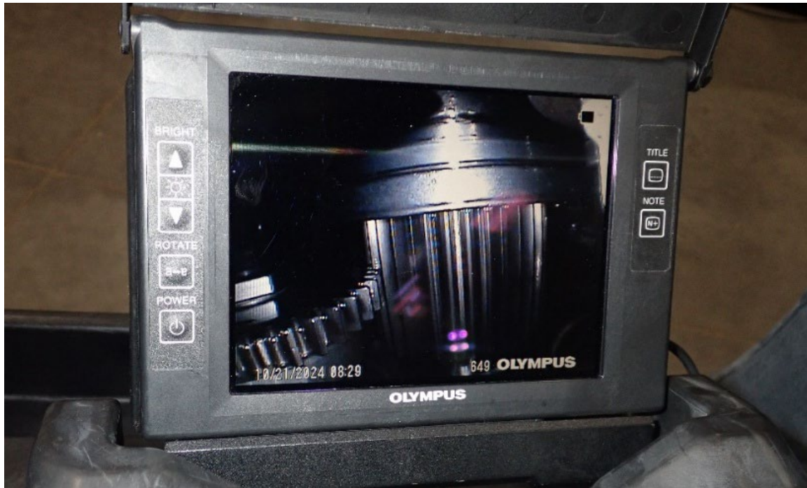
Figure 9. Borescope Image of High-Speed Pinion - Torque Sensor Gear Mesh
