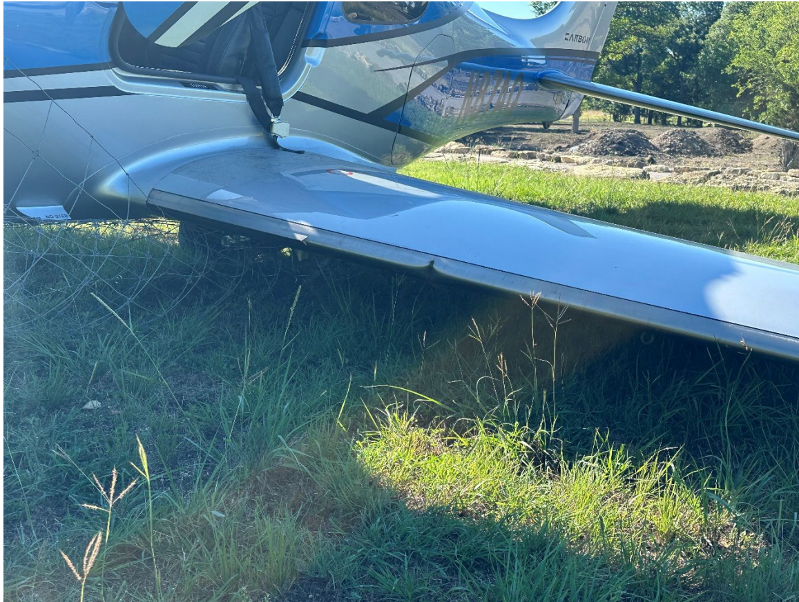
Photograph 3 - Left wing damage (Courtesy of Flight School Manager)
