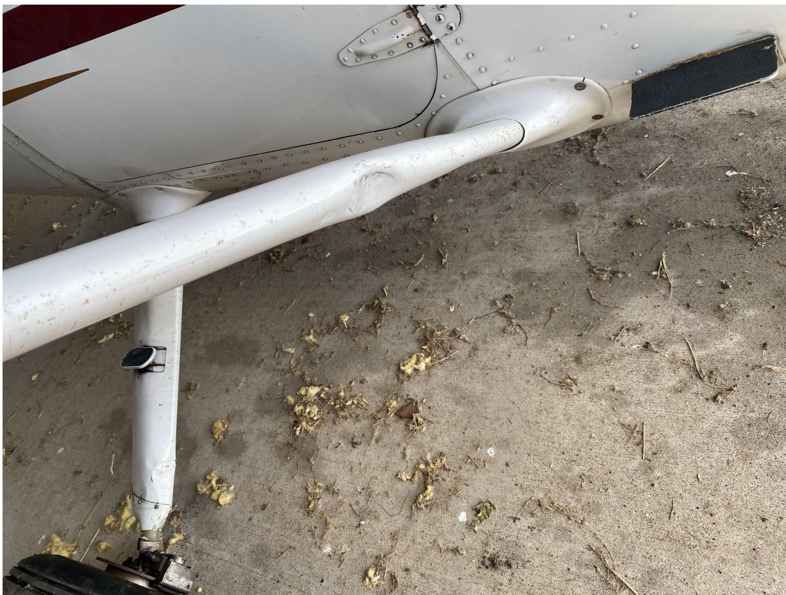
Photograph 1 - Right Lift Strut Damage (Courtesy of Federal Aviation Administration)
