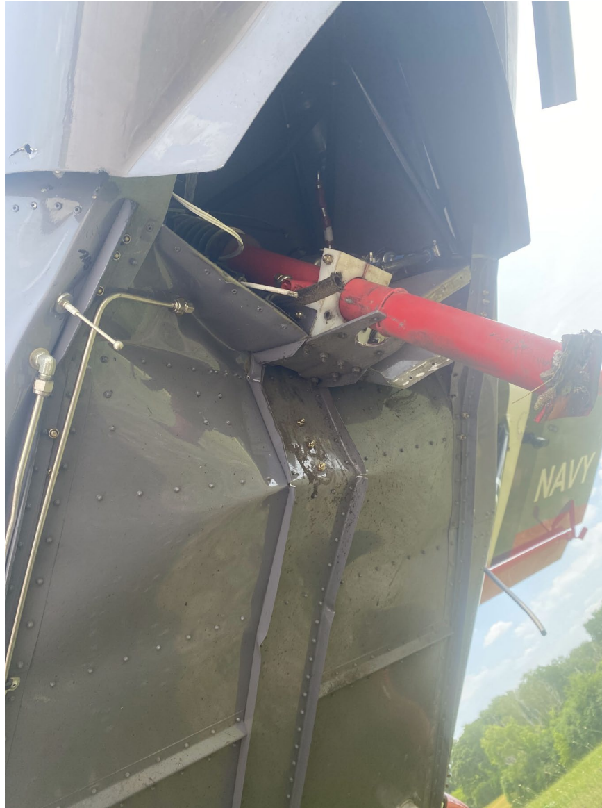
Photograph 4 –Fuselage damage (Courtesy of the pilot)
