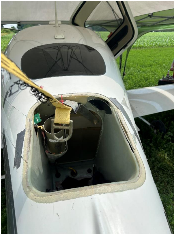
Pic 3: CAPS Rocket/Parachute Exit Cover Area
