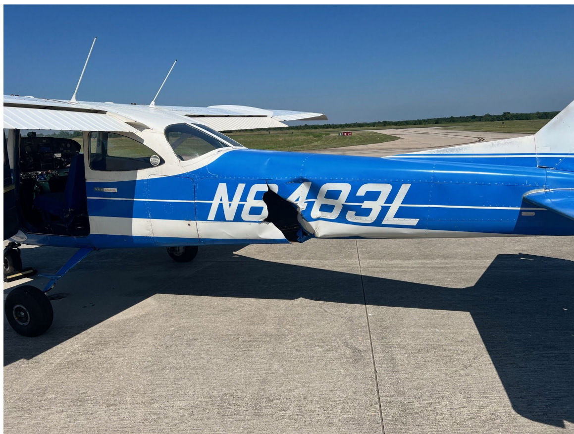
Photograph 1 - View of damage to fuselage (Courtesy of FAA)
