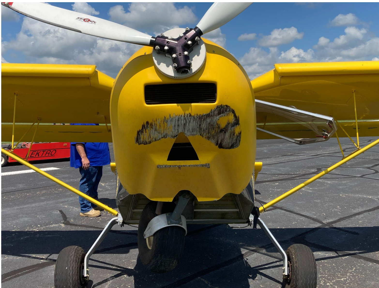
Photograph 2 - Fuselage Substantial Damage (Courtesy of Pilot)
