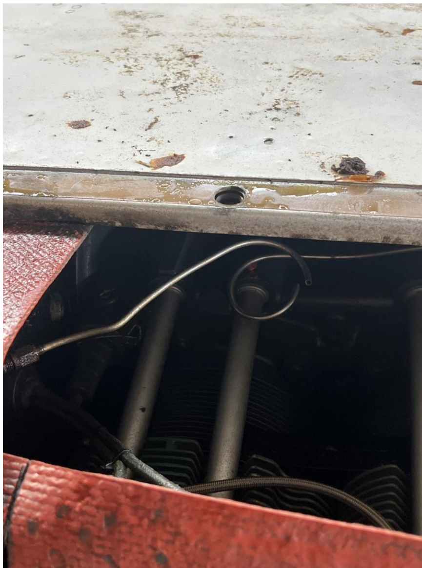
Photograph 6 - Engine Oil Pressure Line (Pilot Photo)
