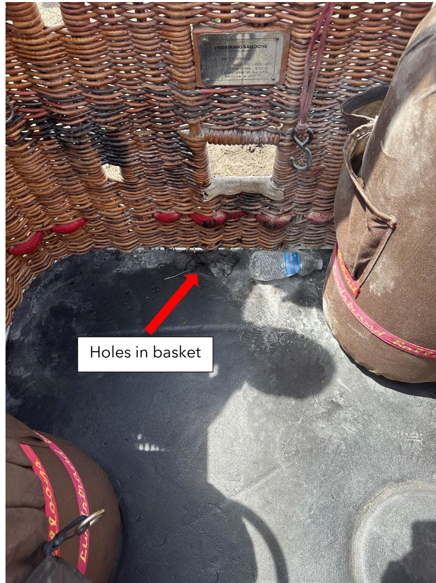
Photograph 1 - Holes burned in the bottom of the basket (Courtesy of FAA)
