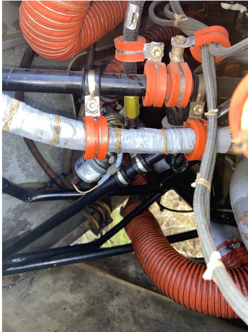
Photograph 4 - Impact damage to engine mount (Courtesy of FAA)
