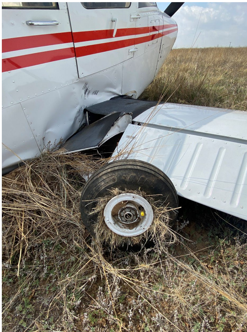
Photograph 2 - Impact damage to right wing & fuselage (courtesy of FAA)
