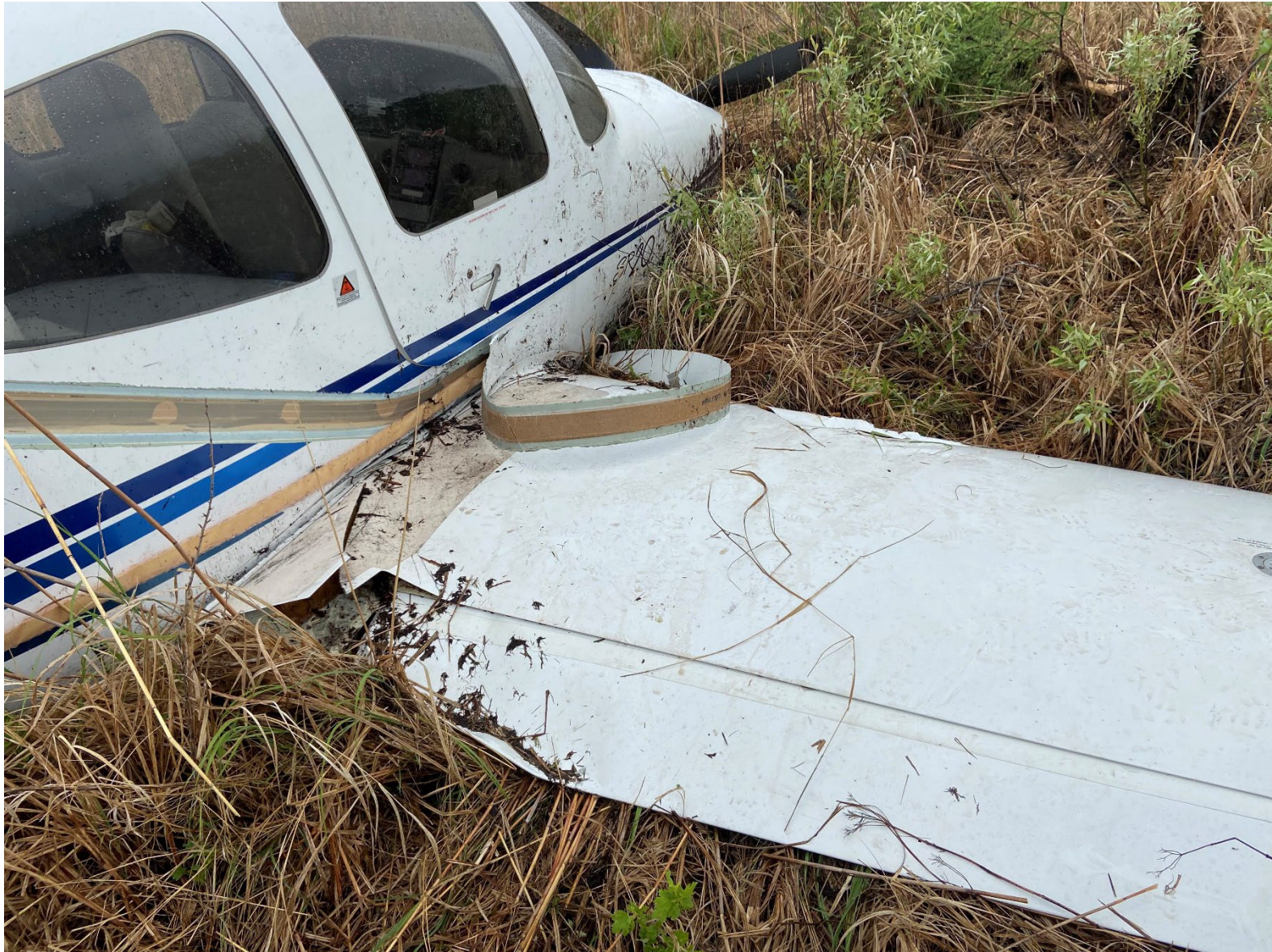
Photograph 2 - Right wing damage (Source: Cirrus Aircraft)
