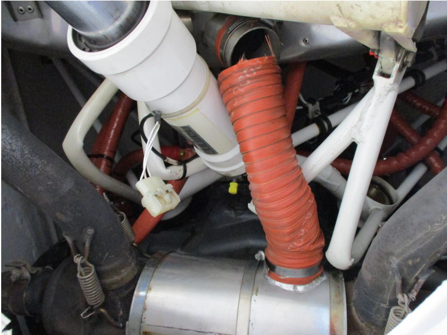
Photo 6 - Damage to engine mount tubes (Courtesy of FAA)
