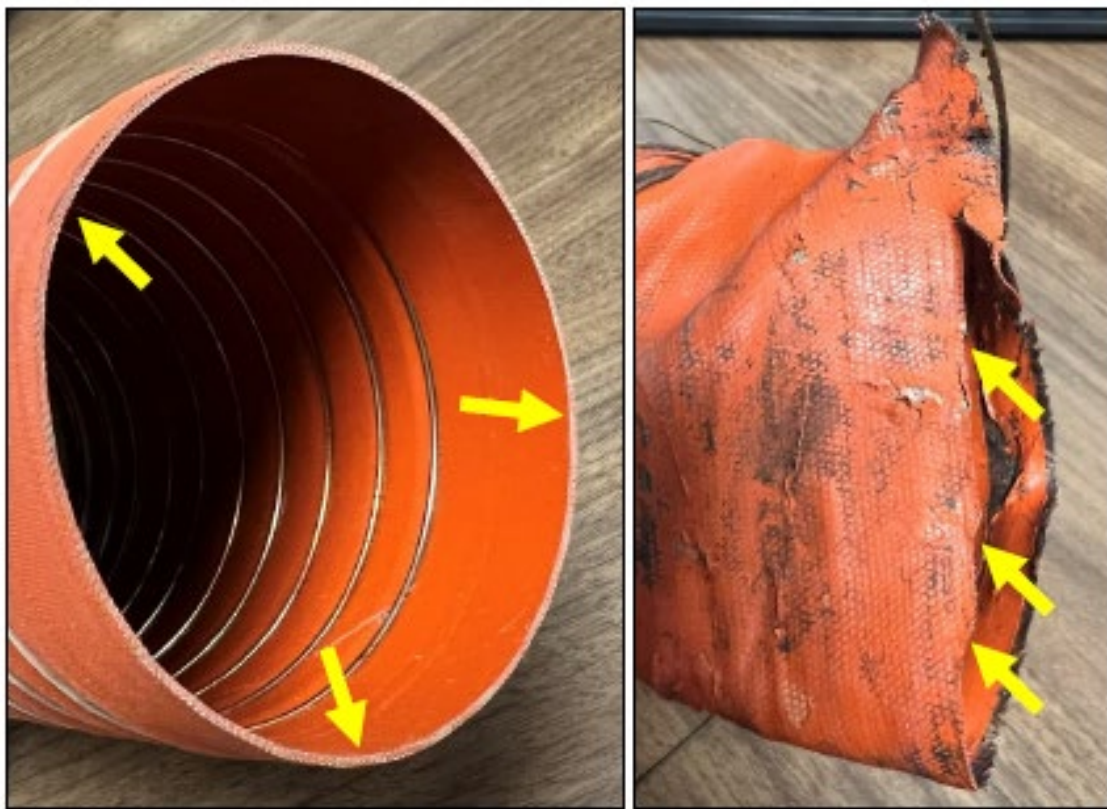
Figure 1 - comparison of stock hose (right photo) to accident airplane's installed hose (left photo). Photo courtesy of Piper Aircraft.
