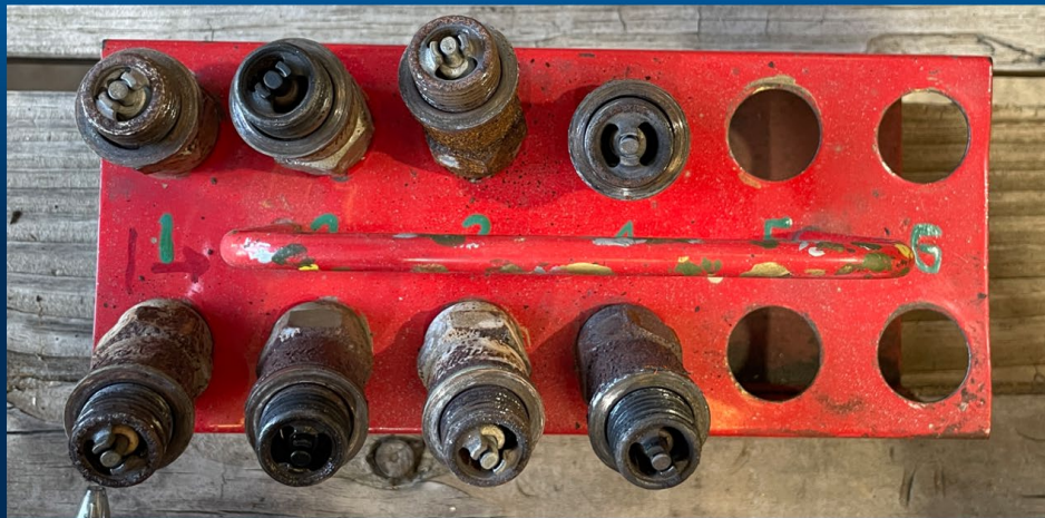
Figure 3 - Spark Plugs Before Engine Runs Conducted
