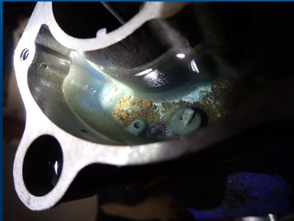
Sediment present in left side of fuel bowl on carburetor.
