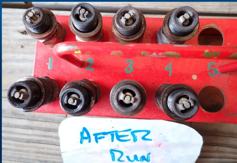
Figure 4 - Spark Plugs After Engine Runs Conducted
