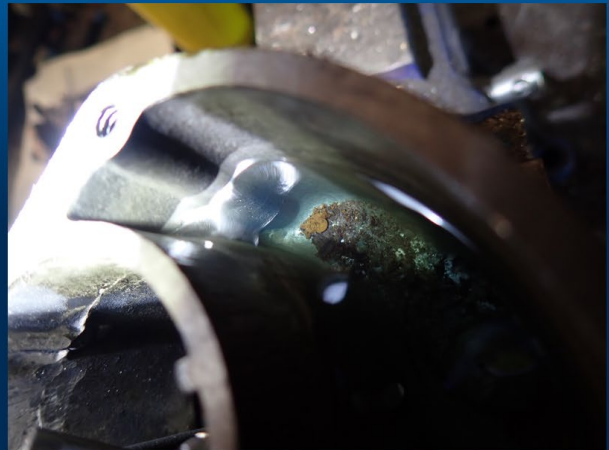
Sediment present in right side of fuel bowl on carburetor.
