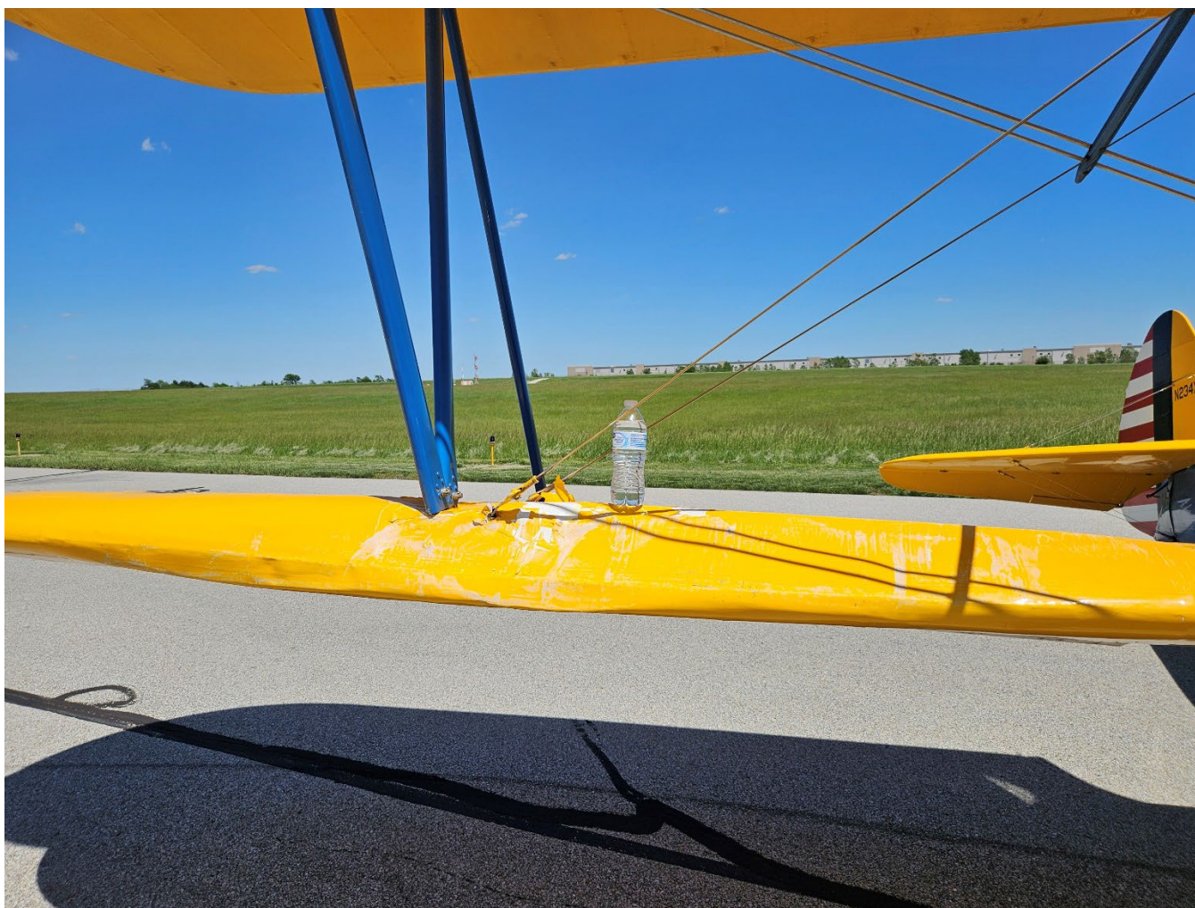
Photograph 2 - Stearman wing damage (Courtesy of FAA)
