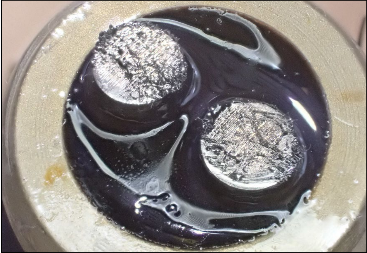
Figure 28: Small metal shavings on chip detector
