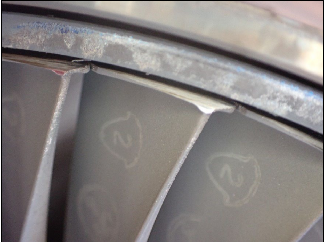
Figure 24: Rubs on the front faces of the blade tip shrouds
