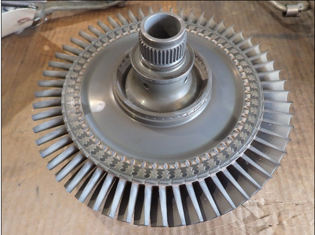
Figure 27: Upstream side of CT disk
