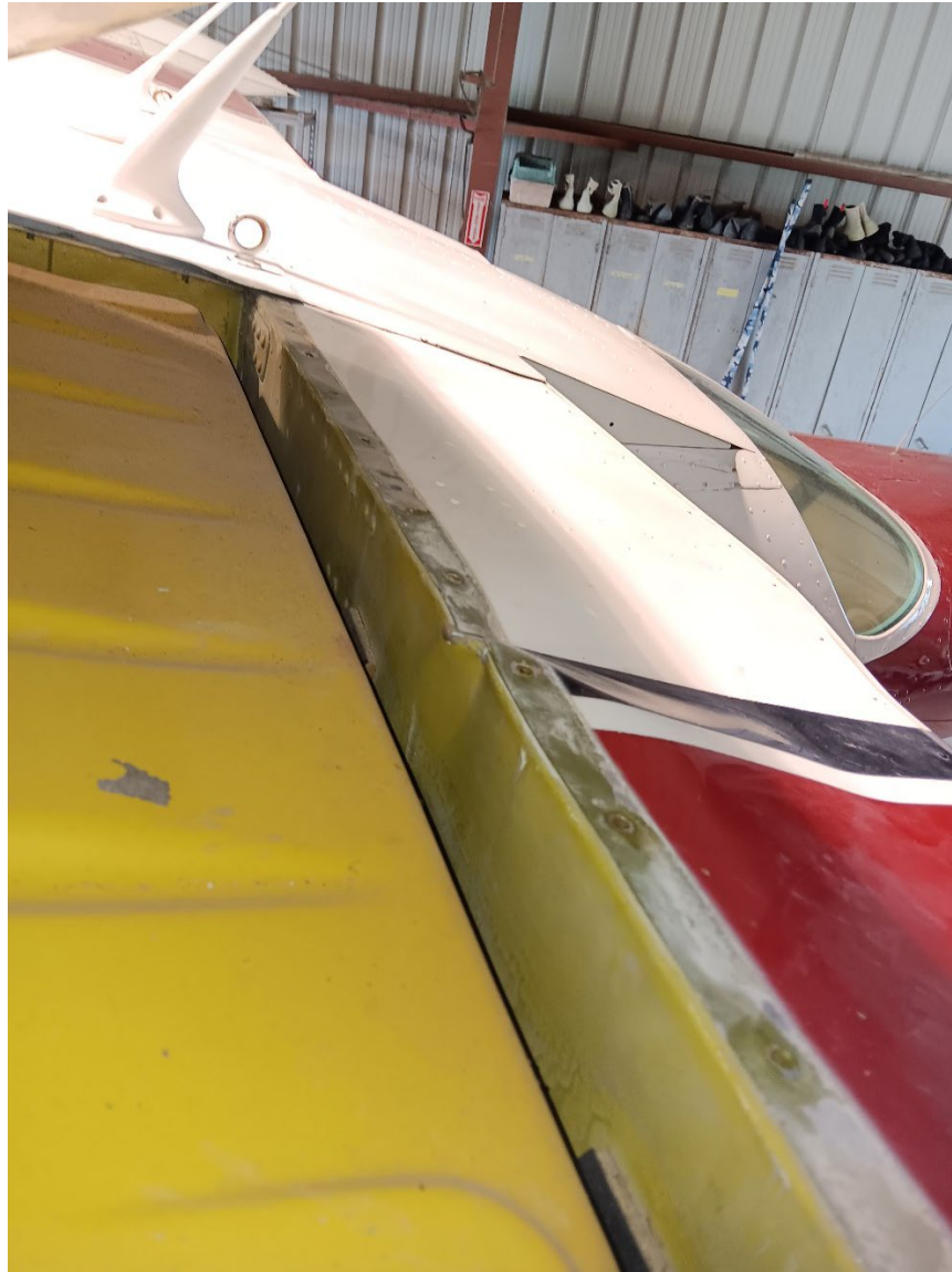
Photograph 1 - N2782L Left Wing Damage (Courtesy of the Federal Aviation Administration)
