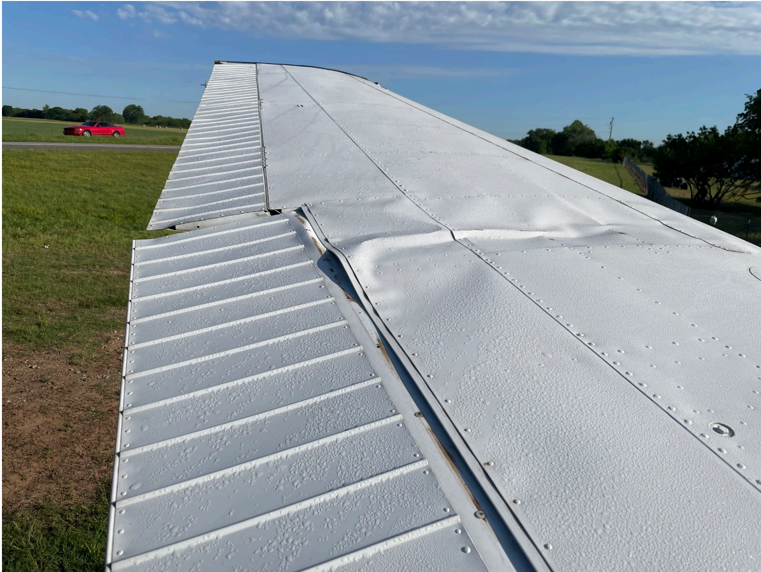
Photograph 3 - Damaged Left Wing (Courtesy of FAA)
