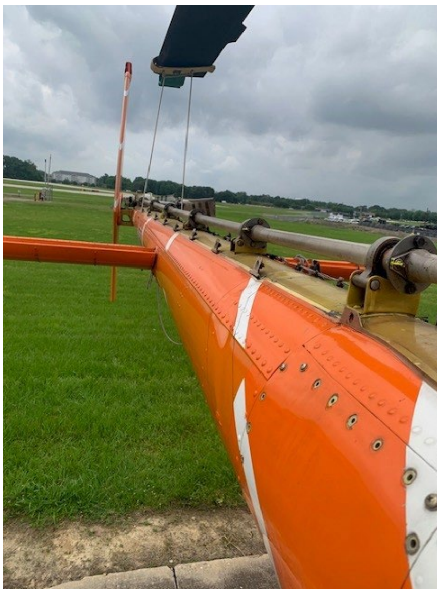
Photograph 2 - Substantial Damage to the Tailboom (Courtesy of FAA)
