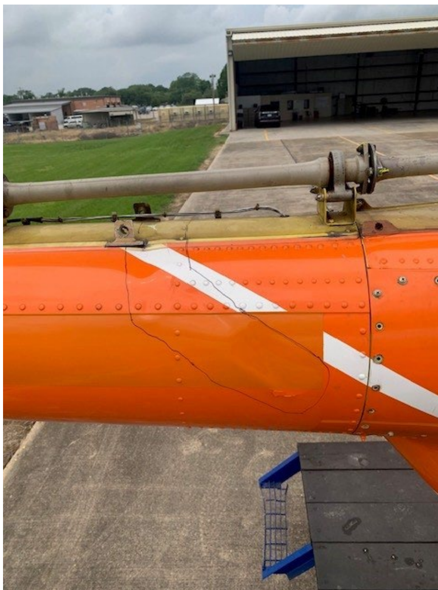
Photograph 3 - Closeup of Substantial Damage to the Tailboom (Courtesy of FAA)
