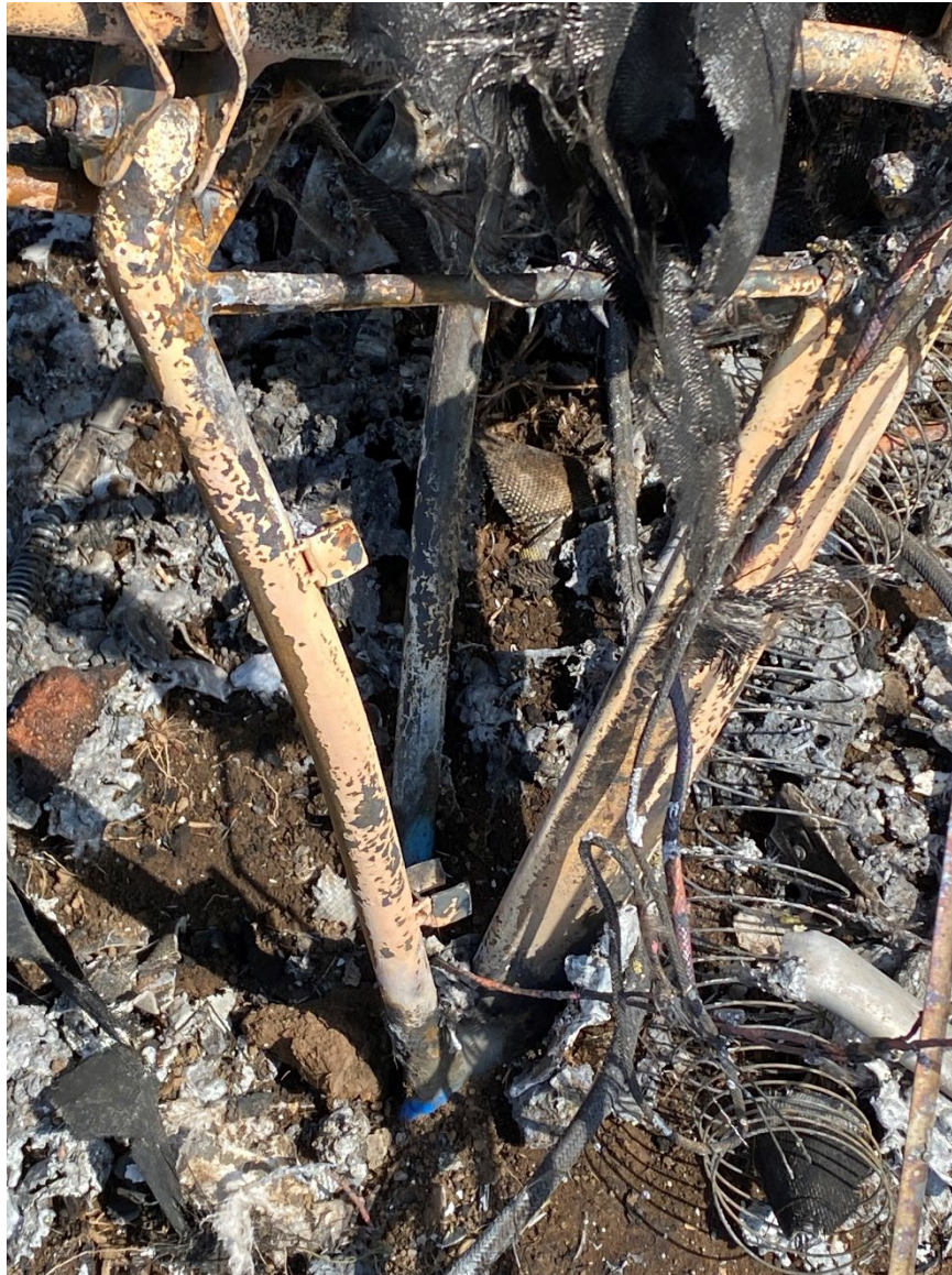
Photograph 3 - Right main landing gear assembly (Source: Federal Aviation Administration)
