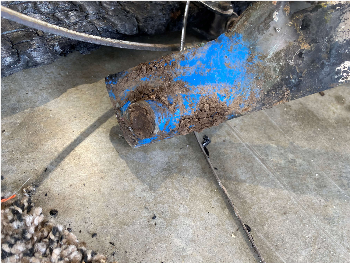
Right gear/frame attachment break point (Part sent to NTSB):
