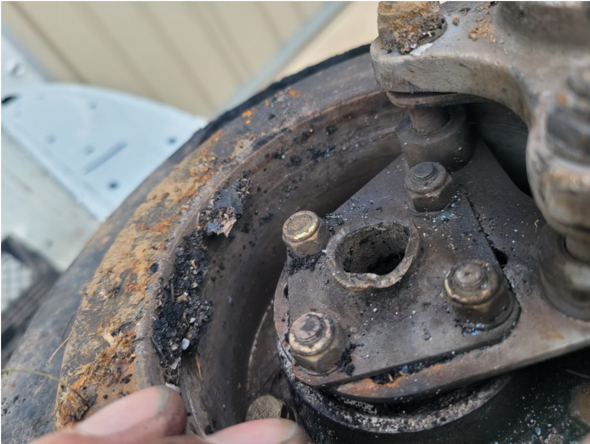
Right Wheel break point showing evidence of prior rust (Part sent to NTSB):
