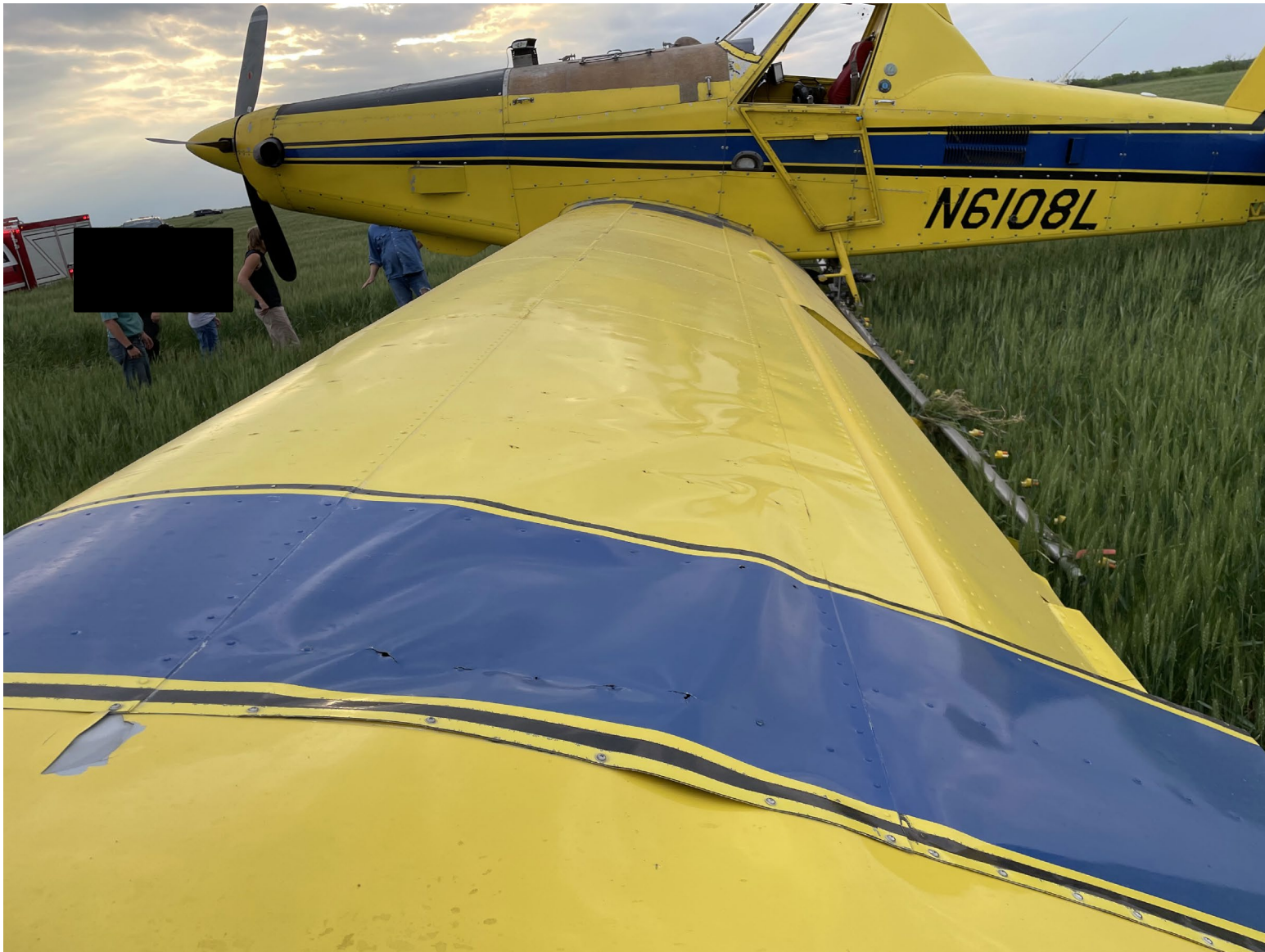
Photograph 3 - Left wing damage (Courtesy of law enforcement)
