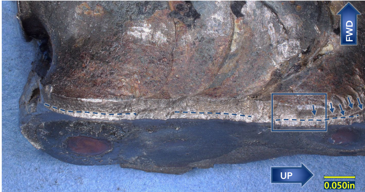
Figure 4. Lower portion of the middle knuckle showing fracture features on the left side. Dashed lines indicate fatigue regions originating at the interior surface, and unlabeled arrows indicate curving crack arrest lines for a fatigue region extending from the weld toe. An SEM image of the area within the rectangle is shown in figure 5.
