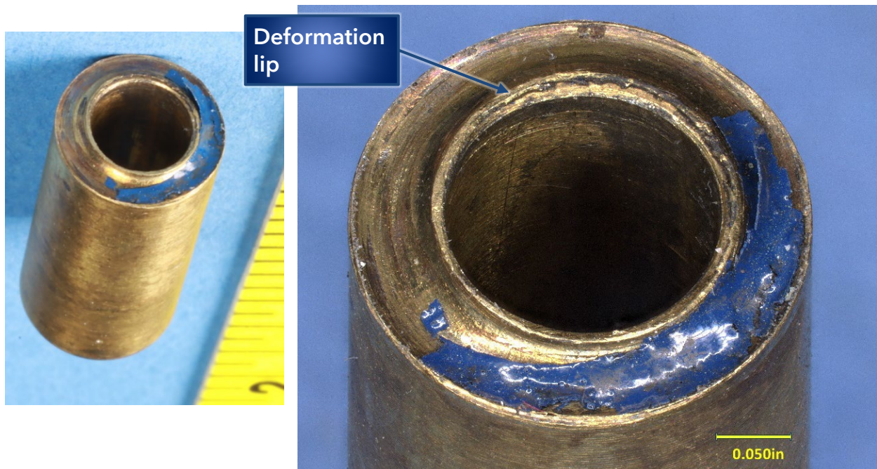
Figure 7. Bushing from the lower hinge with a wear pattern consistent with positioning in the lower knuckle attached to the vertical stabilizer. The lower image shows a closer view of deformation, wear, and paint deposits at one end of the bushing.
