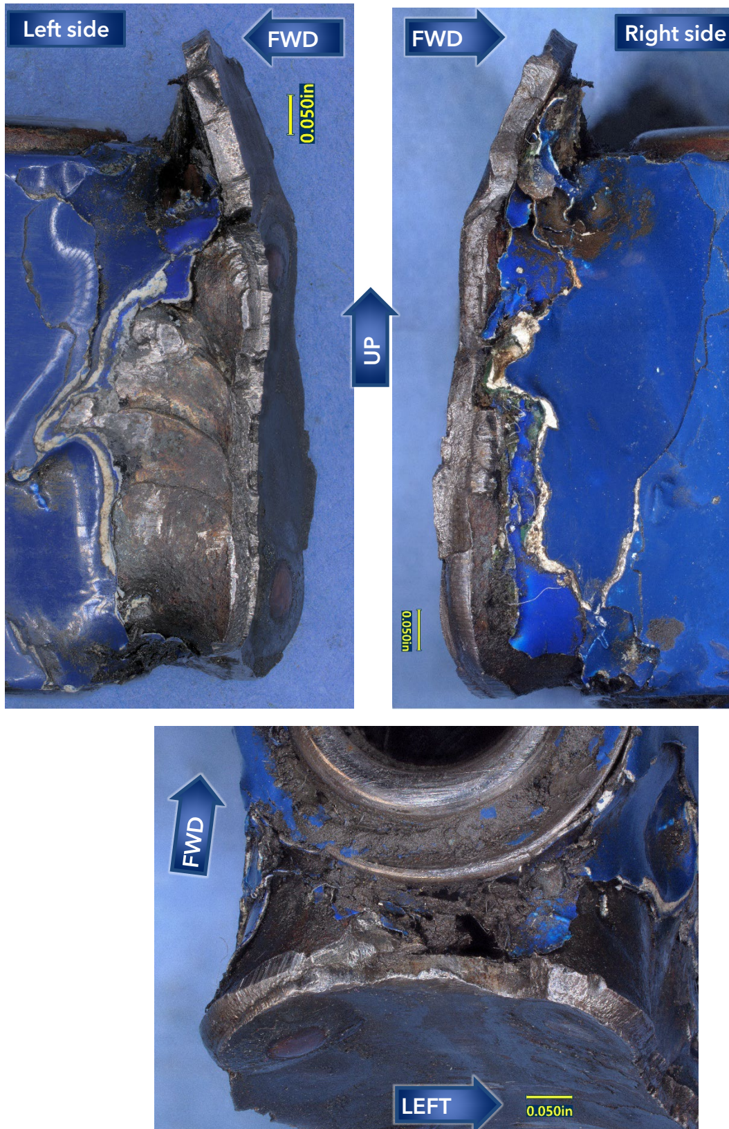
Figure 2. Knuckle side of the rudder post fracture surfaces as received showing the left, right, and lower sides (upper left, upper right, and lower images, respectively).
