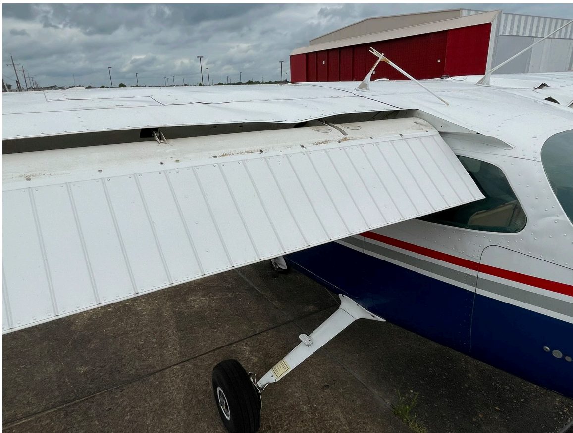
Photograph 2 - Deformation noted to the left and right wings (Courtesy of FAA)
