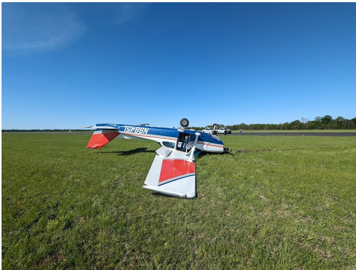
Photograph 1 - Deformation noted to the vertical stabilizer (Courtesy of Airport Manager)
