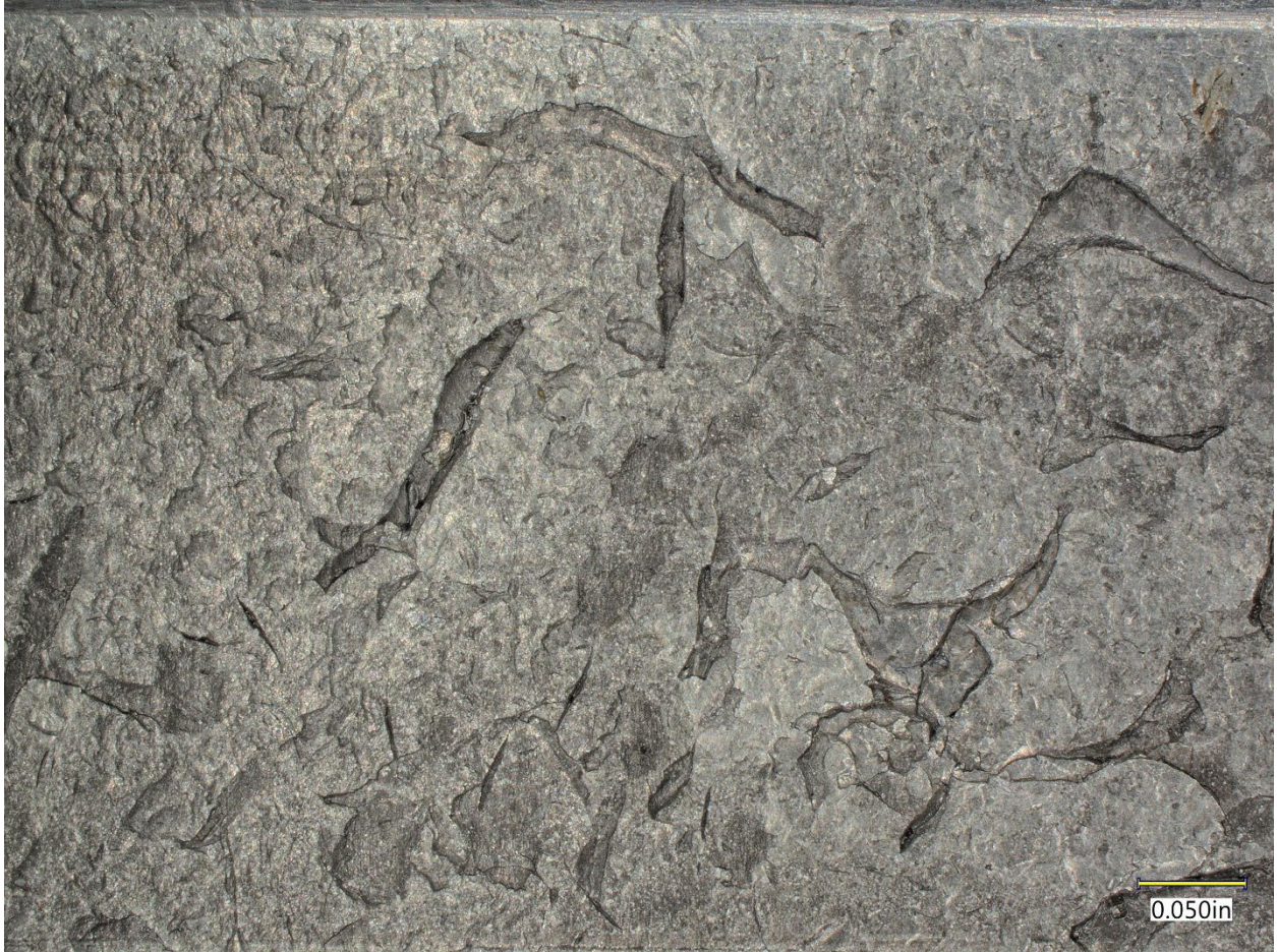
Figure 33. Spalling damage on the ID surfaces of the C4 bearing from Figure 31a.
