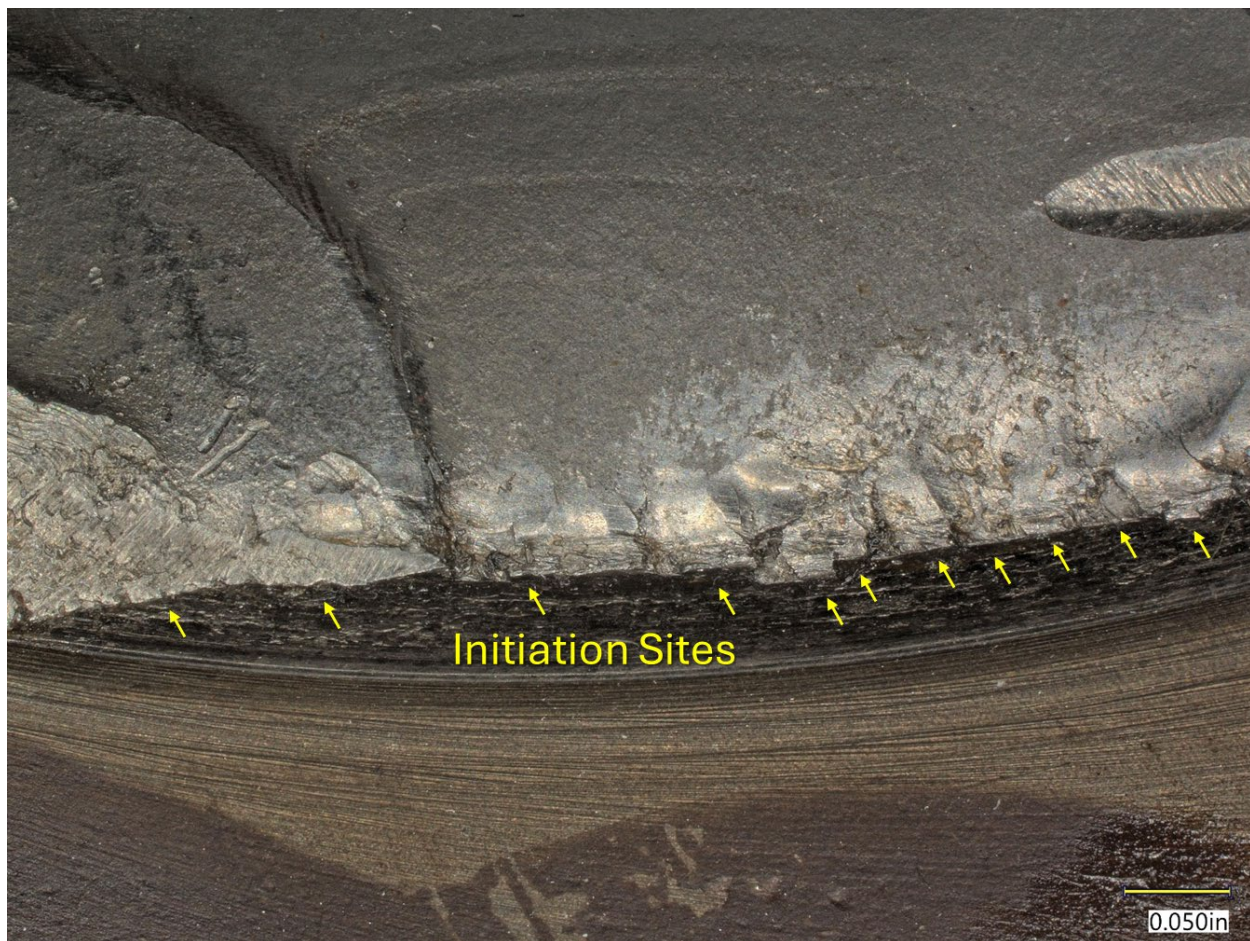
Figure 9. The initiation sites and ratchet marks on the edge of the crankshaft web fracture between the M3 and C4 journal, from the radius with the C4 journal (forward face).
