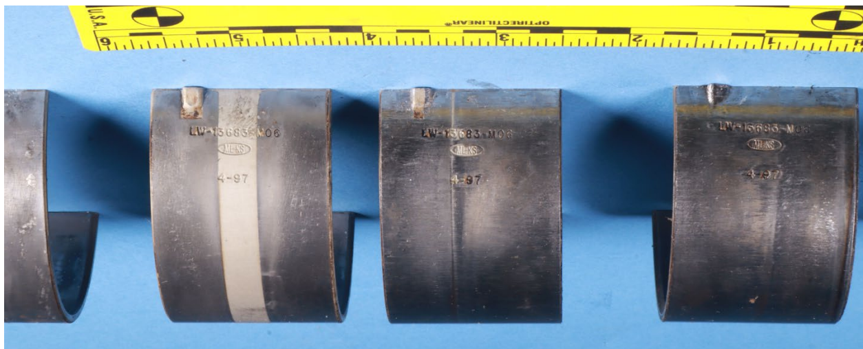
Figure 23. Outer surfaces of several of the other main journal bearings, showing markings stating "LW-136830-M06" and "4-97."
