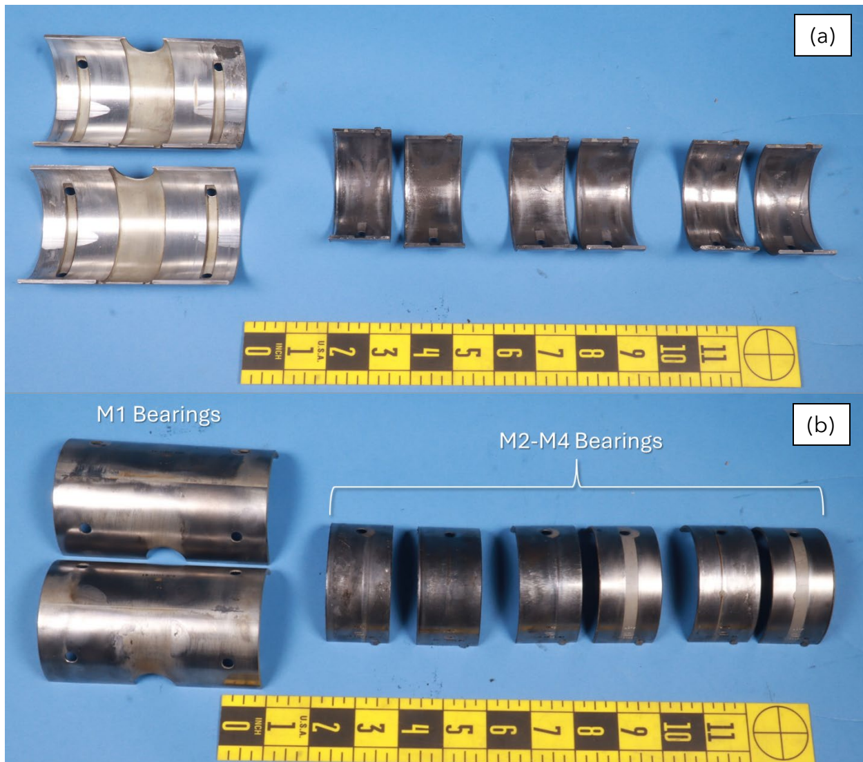
Figure 21. The main bearings, showing the (a) the interior and (b) the exterior surfaces.
