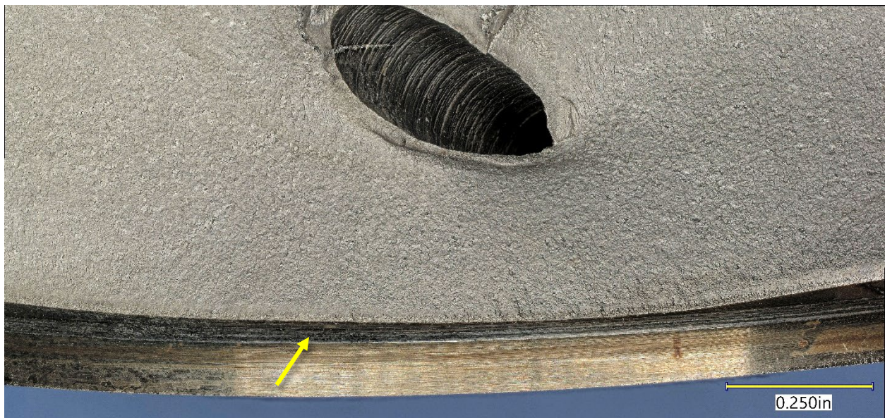
Figure 6. Montage image of the crack initiation site of the M2 fracture surface (yellow arrow).
