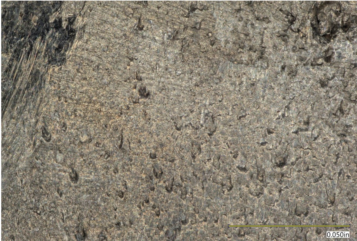
Figure 29. Closer view of the crack arrest marks from the lower left of Figure 28.
