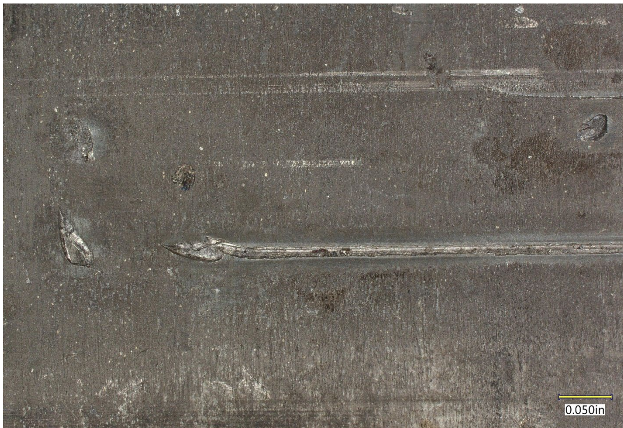
Figure 24. Spalling of the interior surface of one of the main bearings, with a gouge and abrasion marks in the direction of rotation.
