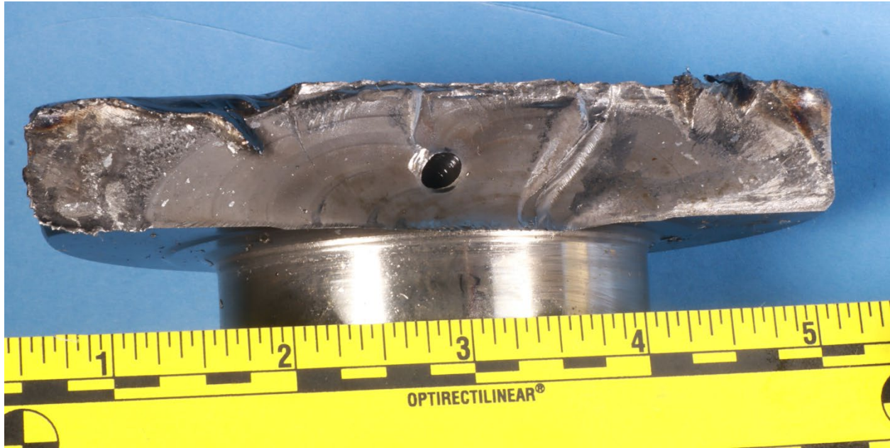
Figure 3. The fracture surface of the crankshaft web between the M3 and C4 locations, viewed from the C4 (aft) side.
