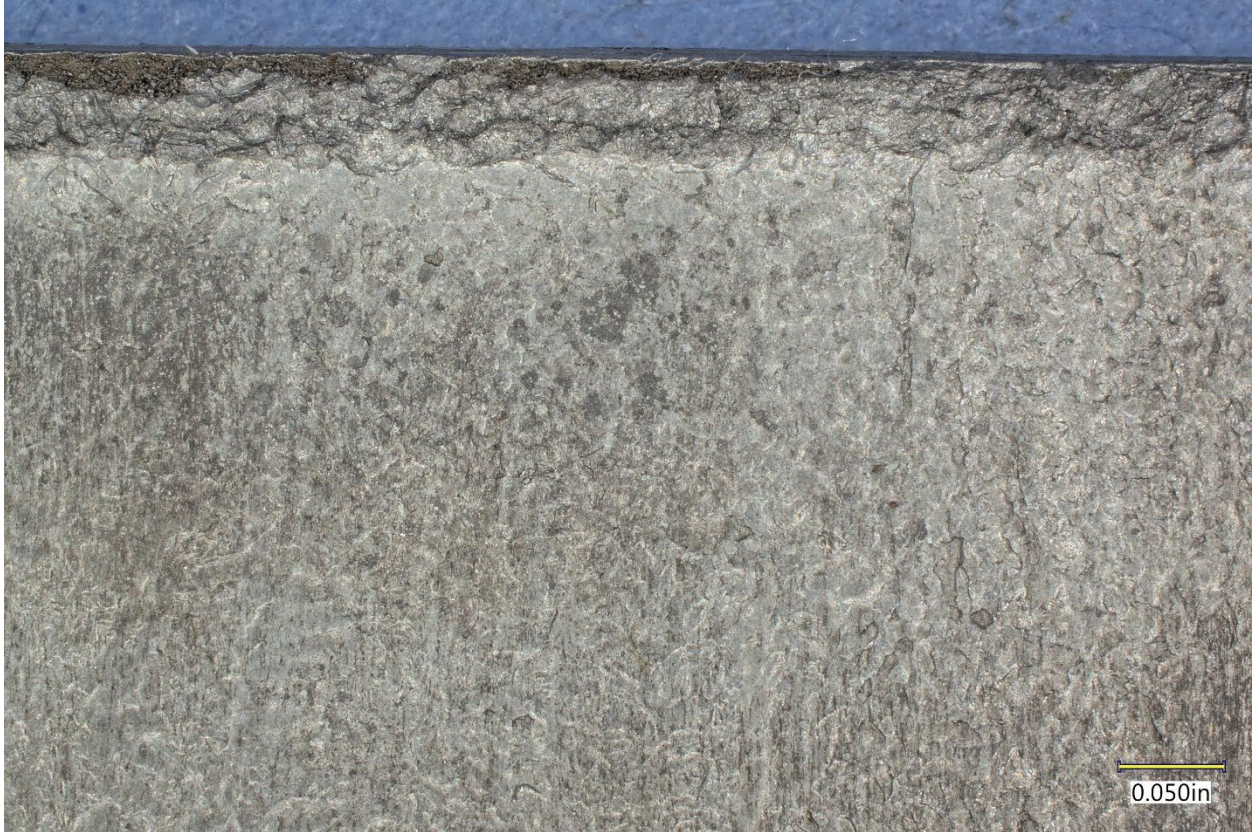
Figure 25. Edge damage, abrasion, and localized spalling on the ID surface of one of the main journal bearings from Figure 23.
