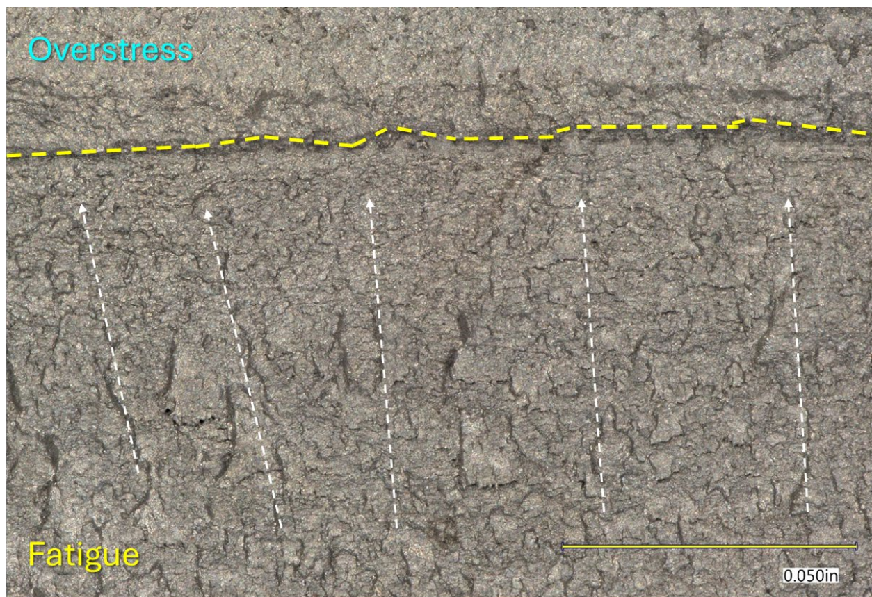
Figure 4. End of the fatigue crack on the M2 web fracture surface.
