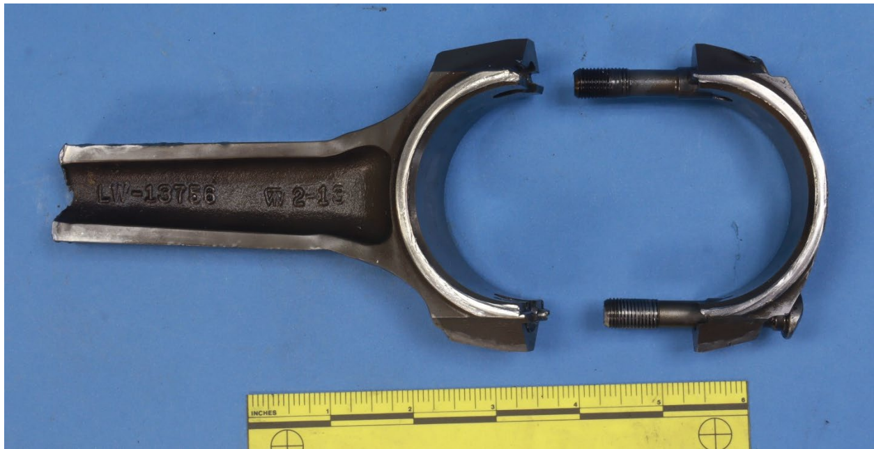
Figure 27. The two halves of the #4 connecting rod, after removal from the crankshaft.
