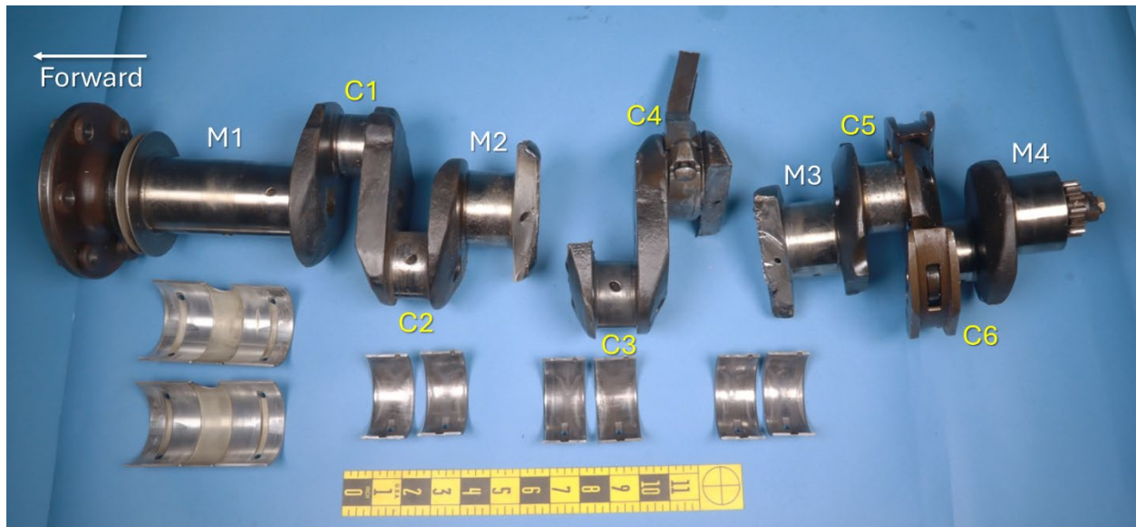
Figure 1. The fractured pieces of the crankshaft, positioned with the bearings, as received.
