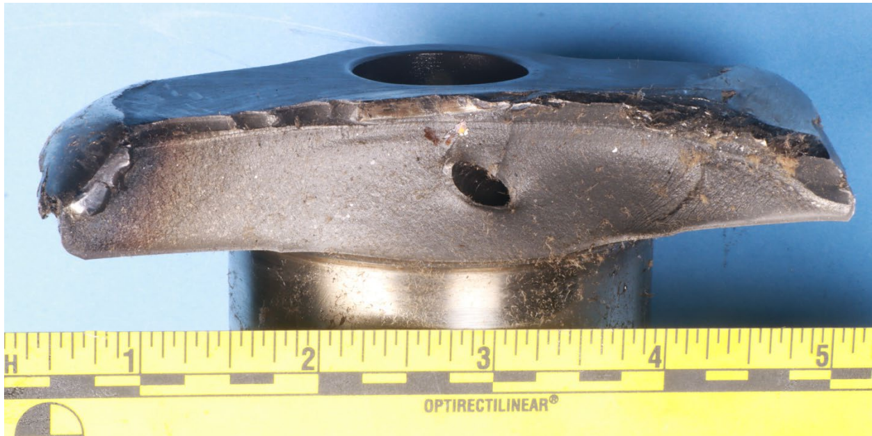
Figure 2. The fracture surface of the crankshaft web between the M2 and C3 locations, viewed from the M2 (forward) side.
