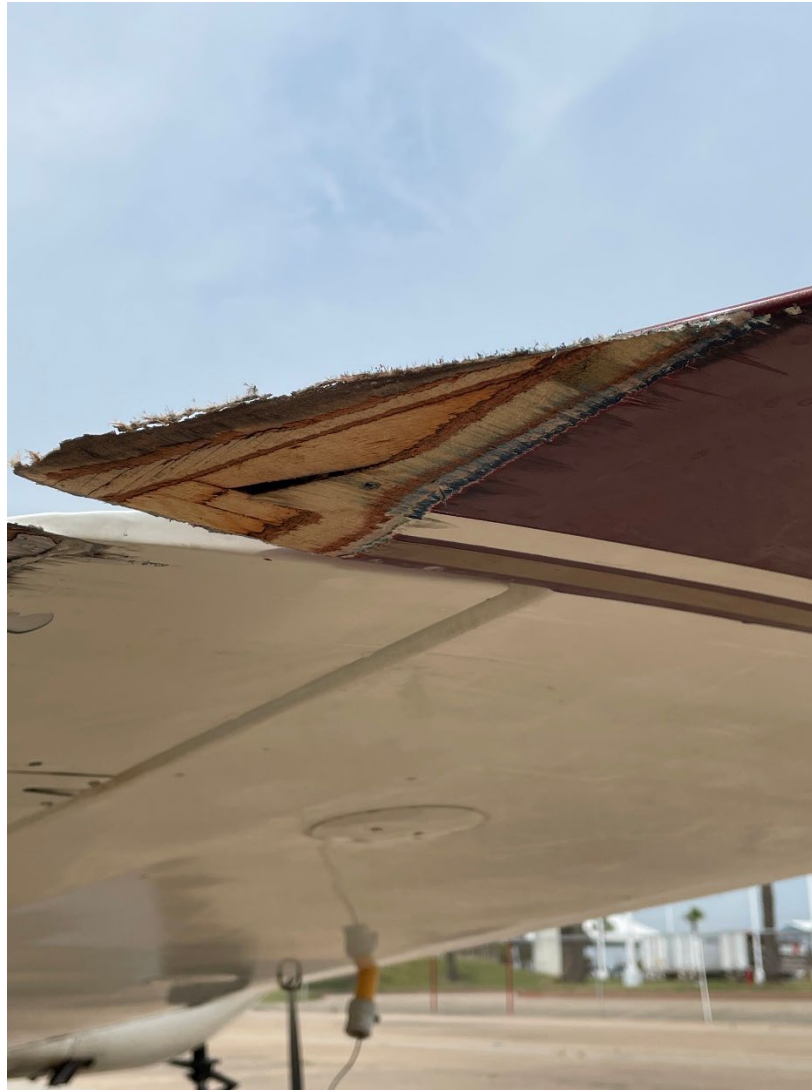
Photograph 4 - Damage present on outboard end of right wing (Courtesy of FAA)
