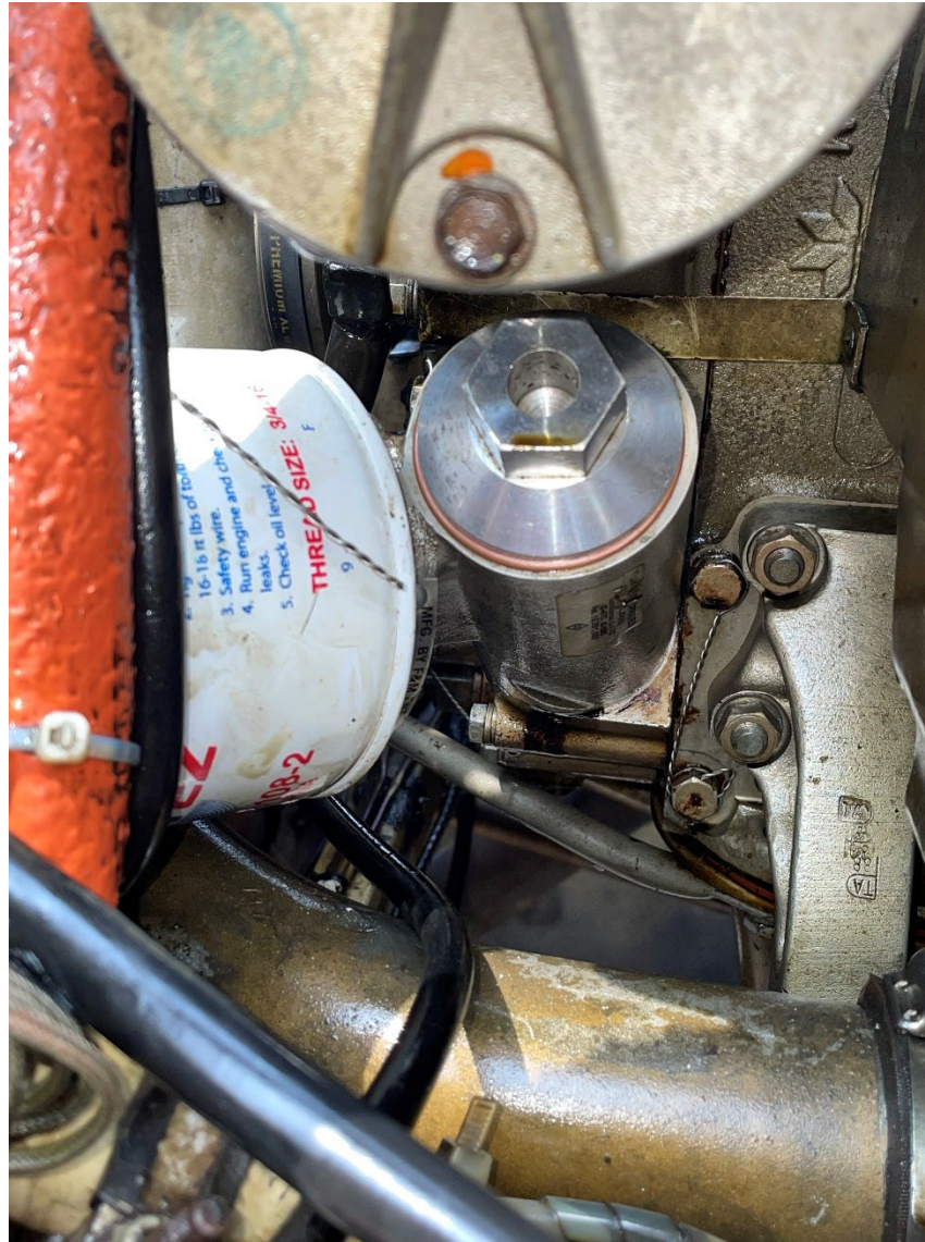
Photograph 2 - Oil filter and oil adapter - note cut safety wire (Courtesy of FAA)
