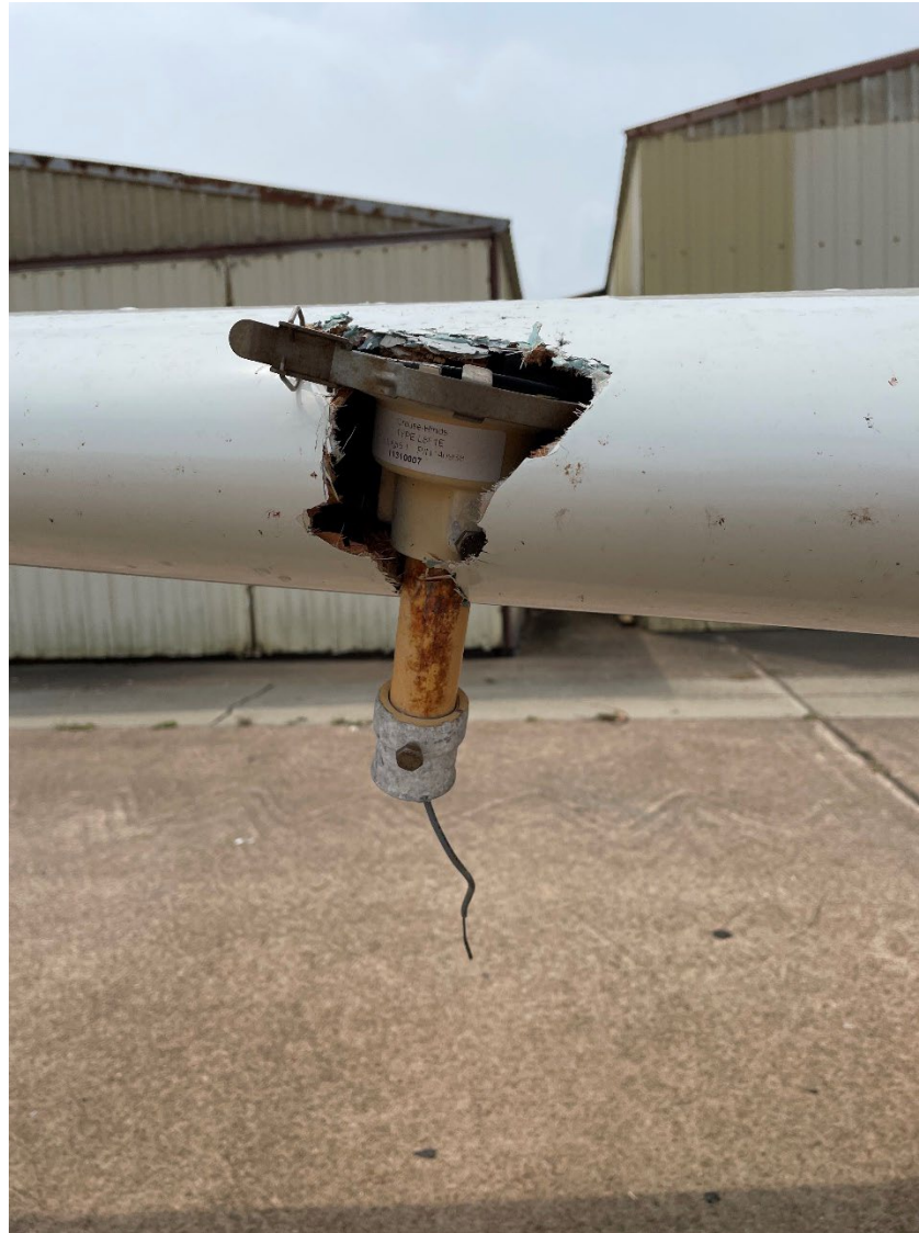
Photograph 3 - Runway light in wing (Courtesy of FAA)
