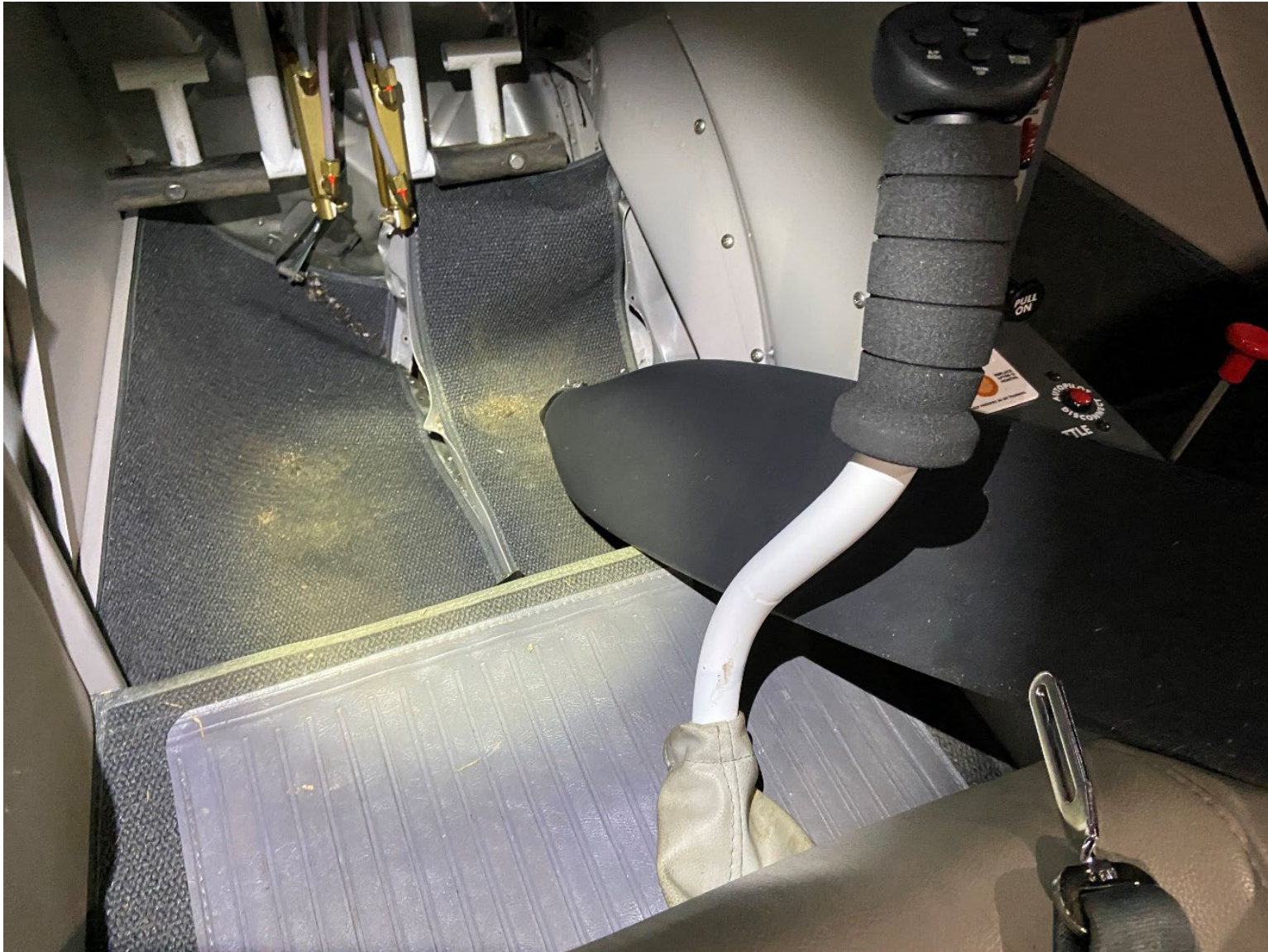
Photograph 5 - View of the substantial damage sustained to the left side cockpit floor (courtesy of the Federal Aviation Administration).
