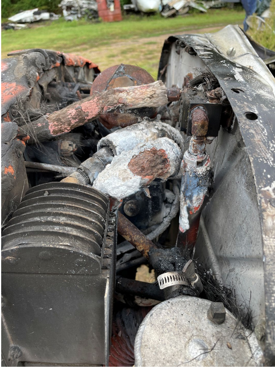
Figure 4. Area between engine and firewall as viewed from left side.
