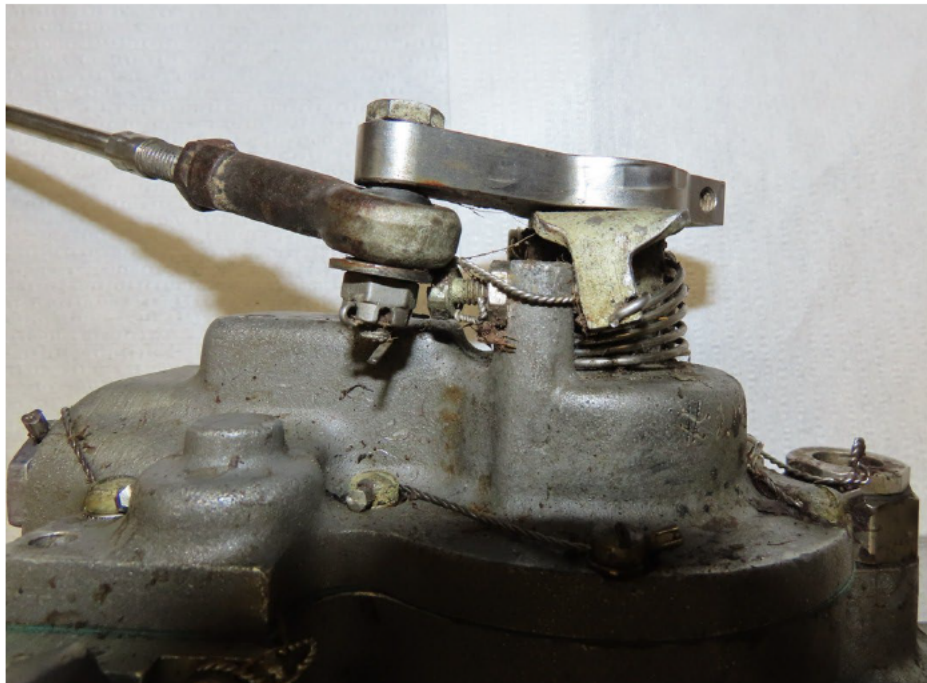
Photo 38- Propeller Governor, Speed Setting Lever Stop Damage
