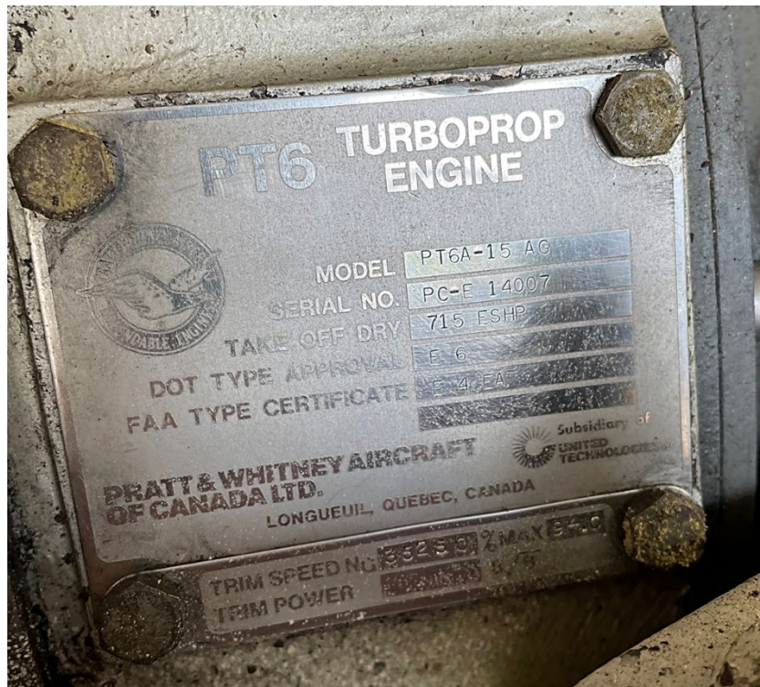
Photo 6- Engine Data Plate
