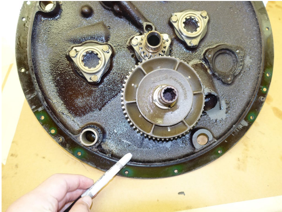
Photo 25- AGB Case Impact Damage, 6 o'clock Position
