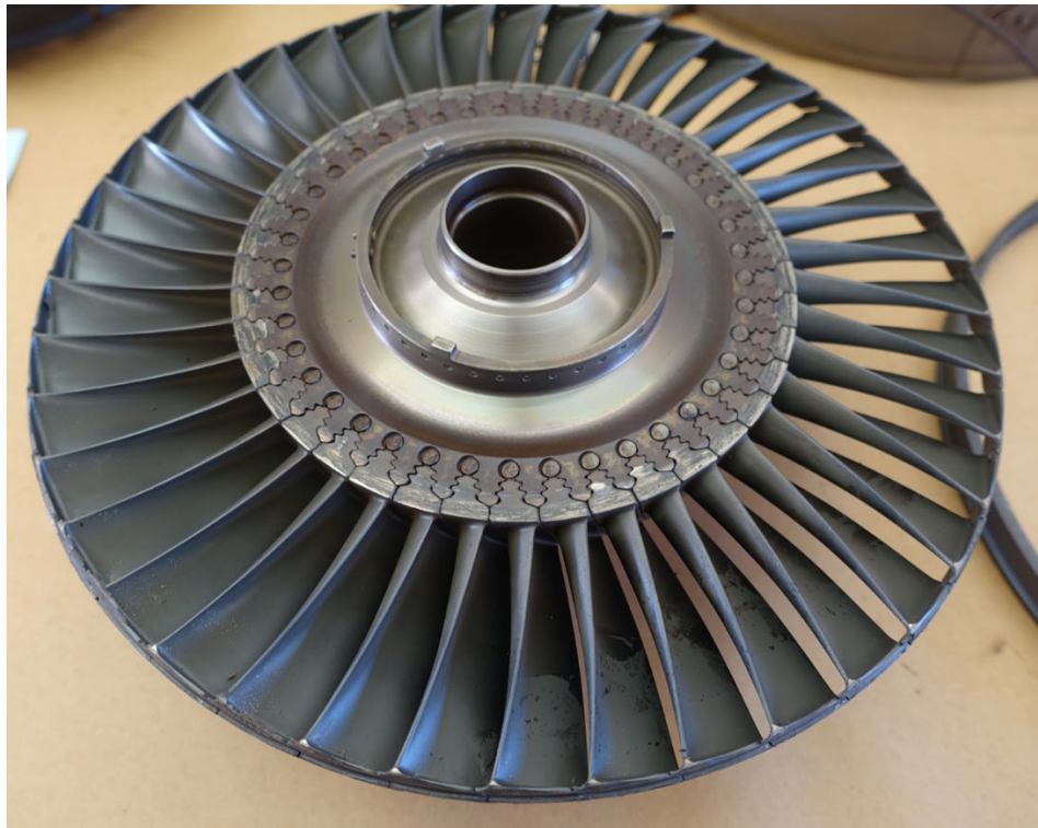
Photo 12- PT Blades, Fir Tree Circumferential Rub
