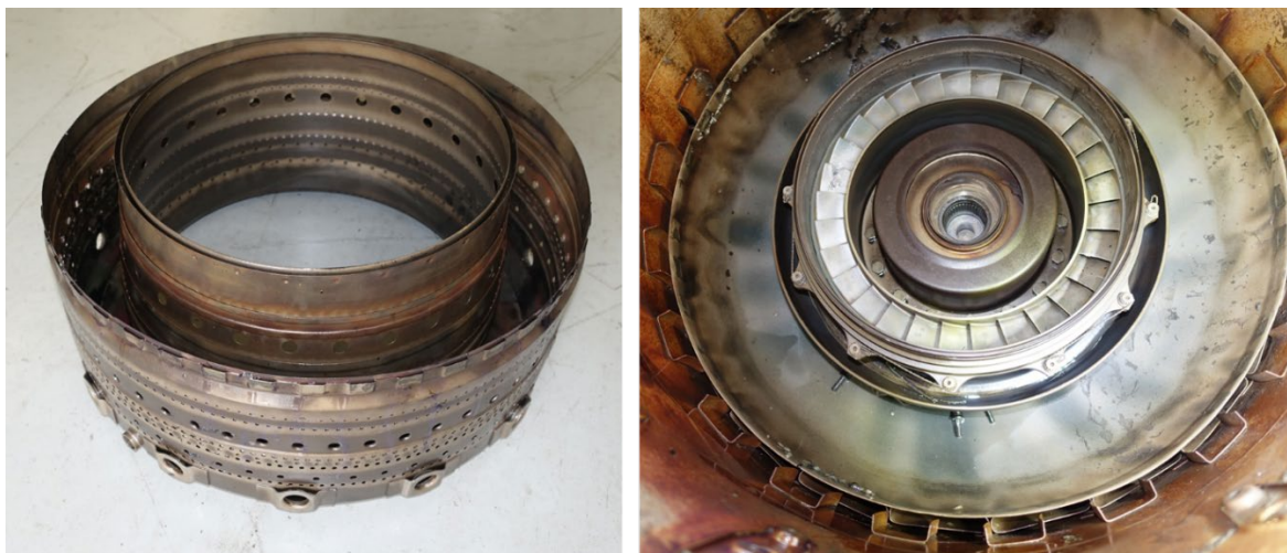
Photo 19- (L) Combustion Liner, (R) Loose Bolts in Large Exit Duct
