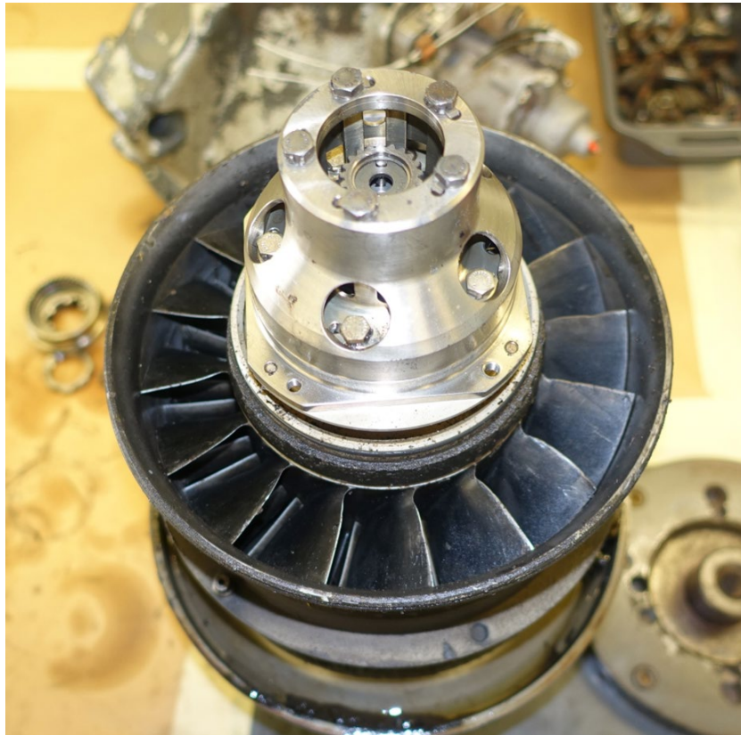
Photo 21- 1 st Stage Compressor Blades
