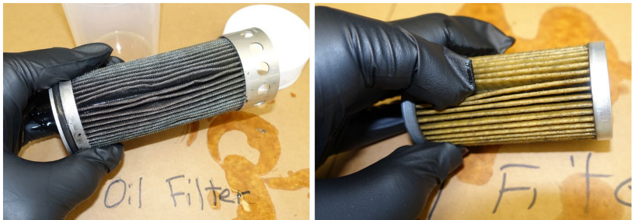
Photo 10- (L) Oil Filter, (R) Fuel Filter
