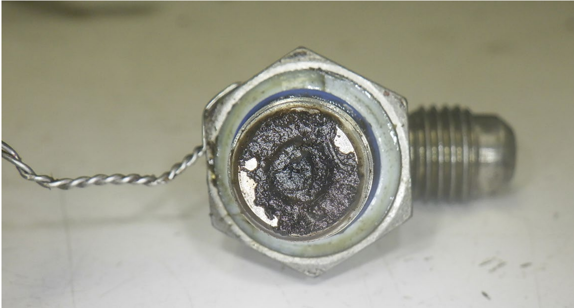
Photo 31- FCU Air Inlet Adapter, Px Fitting Obstruction
