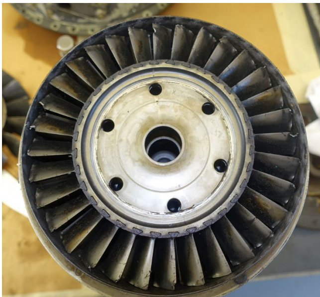
Photo 22- (L) 2 nd Stage Compressor Rotor Blade Damage, (R) 3 rd Stage Compressor Rotor
