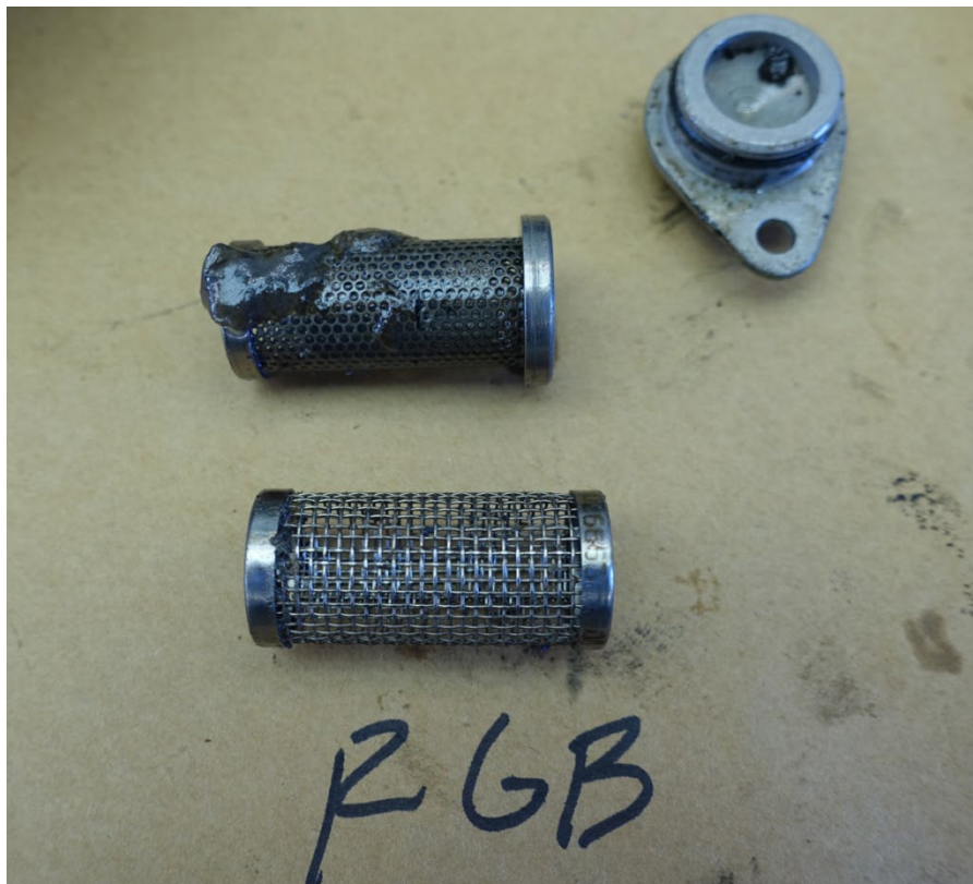
Photo 28- RGB Strainer Screens, (Top) MCD Strainer, (Bottom) Oil Strainer
