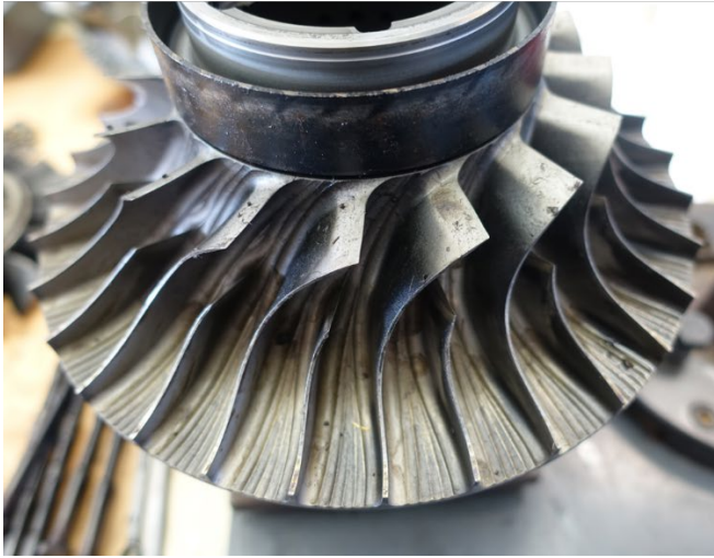
Photo 23- (L) Compressor Impeller, (R) Impeller Shroud
