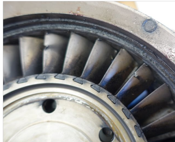
Photo 22- (L) 2 nd Stage Compressor Rotor Blade Damage, (R) 3 rd Stage Compressor Rotor
