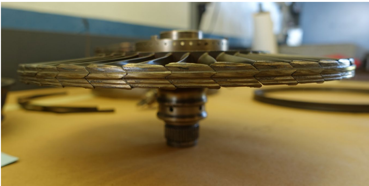
Photo 14- PT Blade Outer Platform Rub
