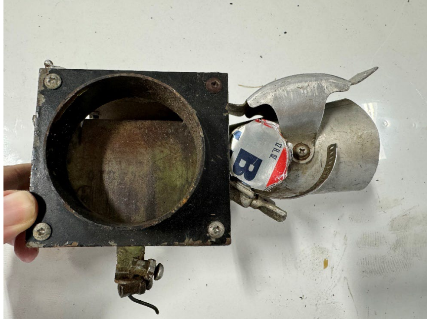
Figure 7. Junction Box with an unapproved part covering the outlet.
