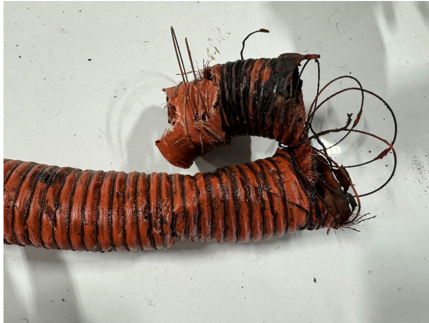
Figure 3. Damaged scat tube.
