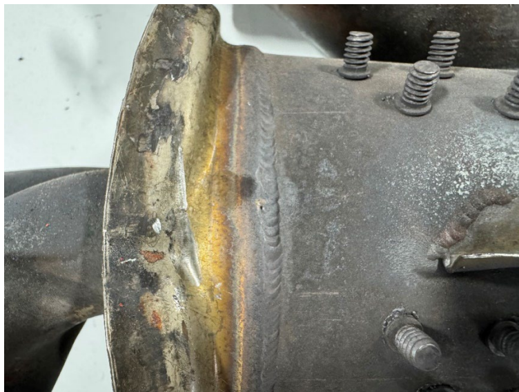
Figure 4. Pin hole in muffler.
