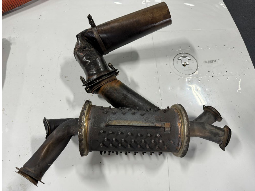
Figure 1. Exhaust System as removed.
