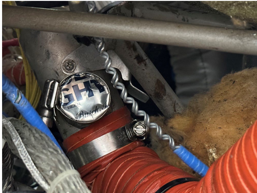
Figure 8. Cabin Air scat tube with an unapproved part covering the inlet.
