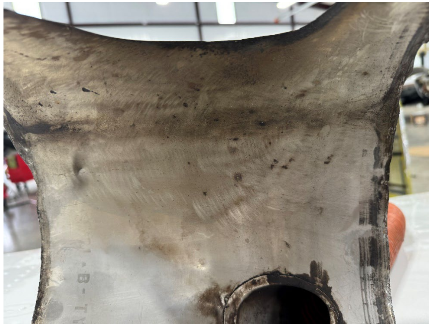
Figure 2. Muffler Cabin Heat Shroud with area of exhaust blowby.
