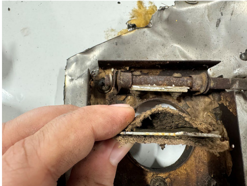
Figure 9. Valve plate and base fracture surfaces.
