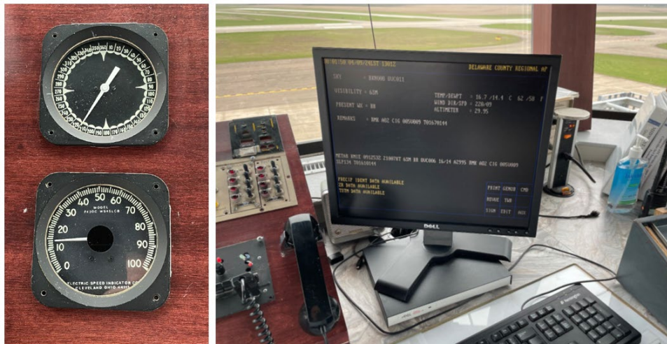
Figure 6 - Photo of tower wind gauge (left) and the ASOS OID display (right) in the KMIE tower.
