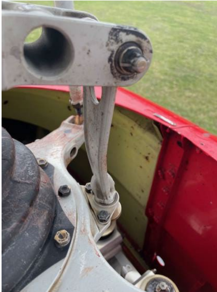
Photograph 3 - Bent swashplate drive link (Courtesy of pilot)
