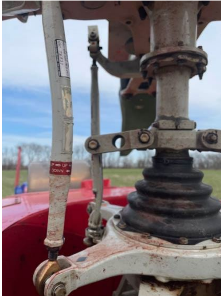
Photograph 2 - Bent pitch change link (Courtesy of pilot)
