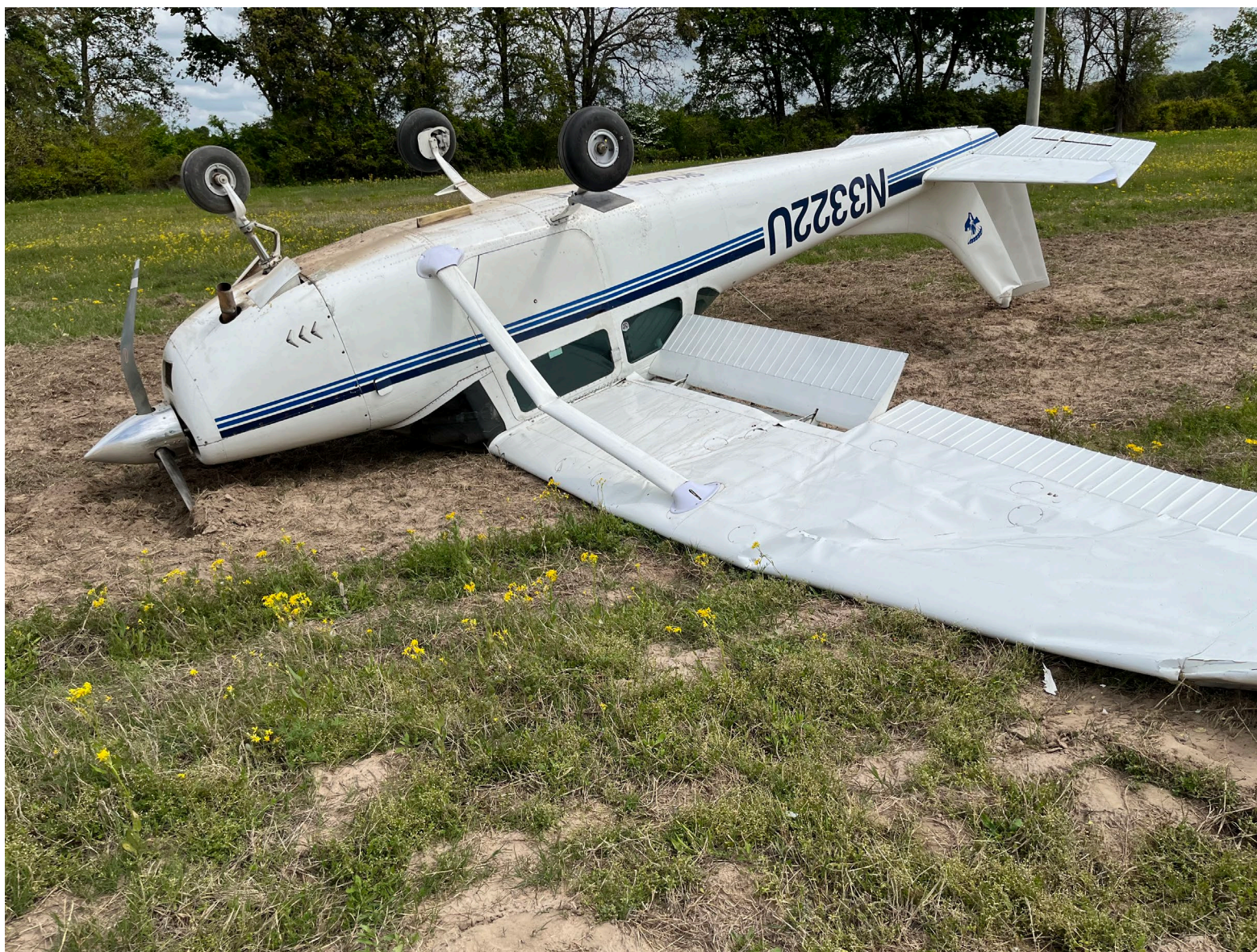
Photograph 3 - Damaged right wing (Courtesy of FAA)
