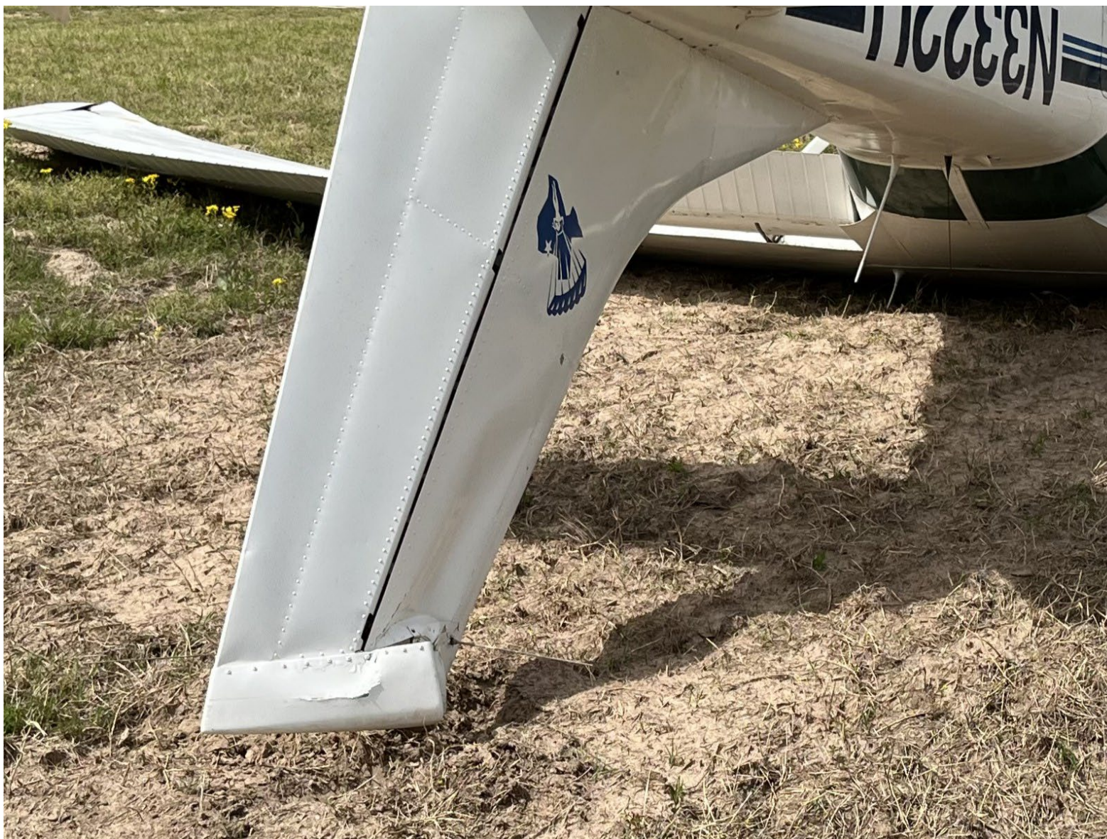
Photograph 2 - Damaged rudder (Courtesy of FAA)
