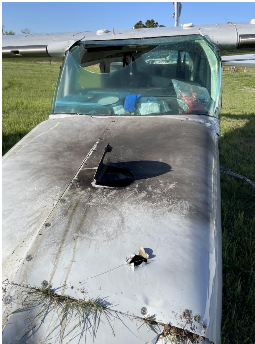
Photograph 3 - Cowling damage (Courtesy of FAA)
