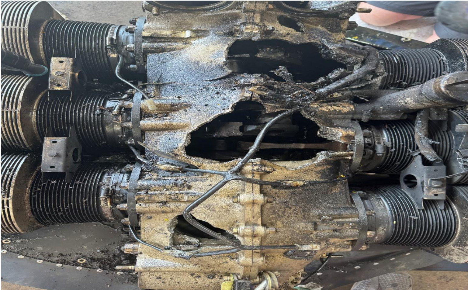
Photograph 6 - Damage to Engine (Courtesy of FAA)
