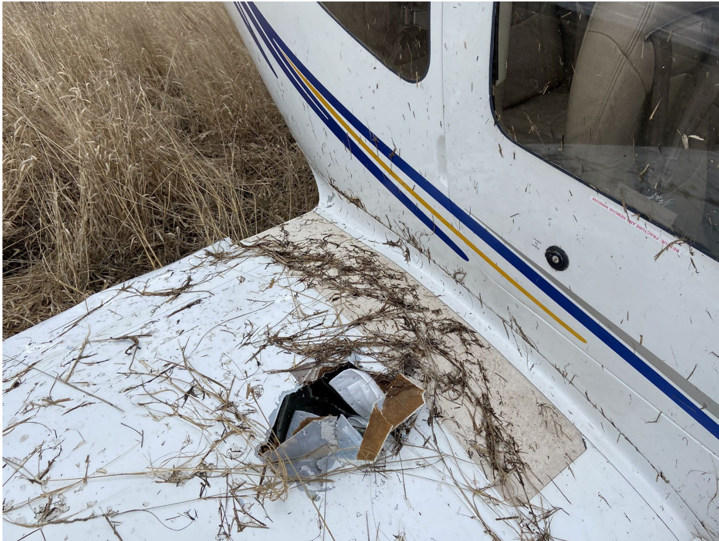
Photograph 2 - Right wing damage (Source: Federal Aviation Administration)
