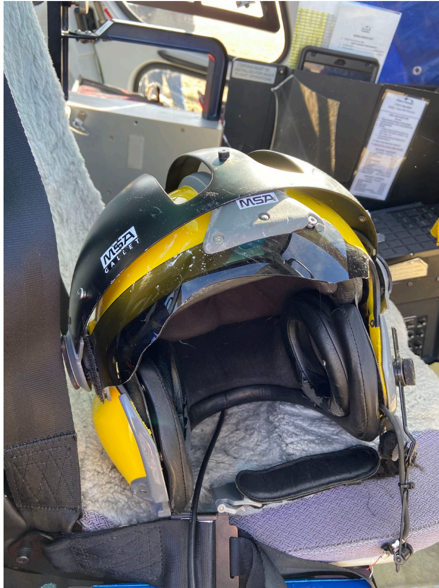
Photograph 3 - Pilot's Helmet Damage (Courtesy of Federal Aviation Administration)
