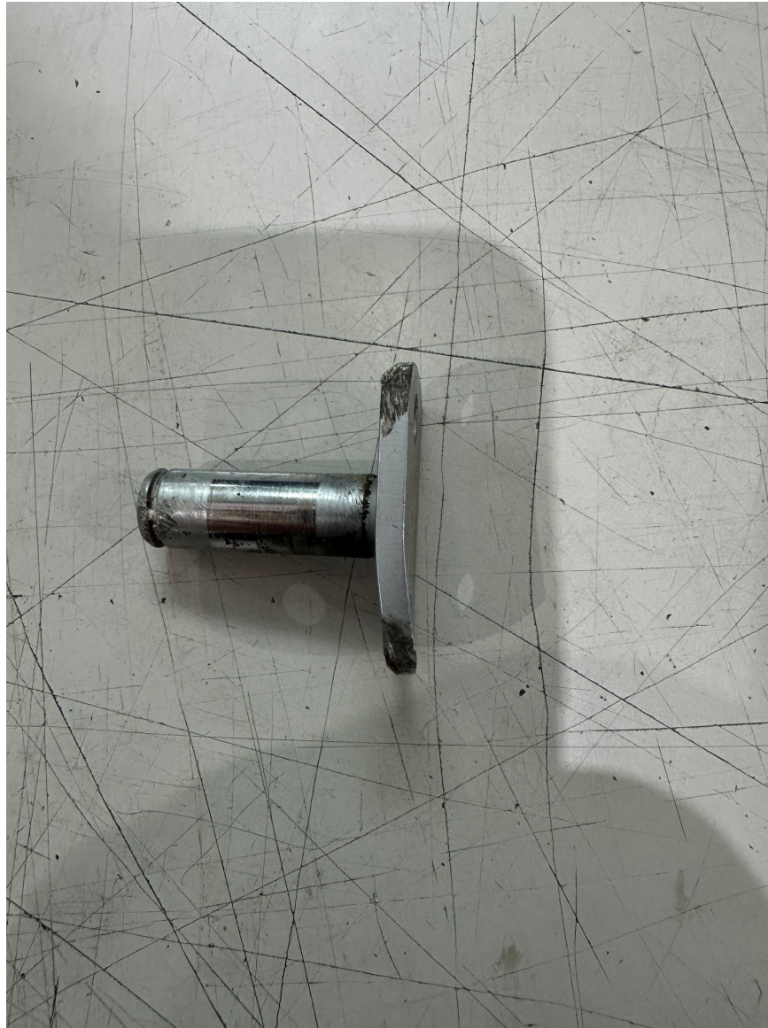
Photograph 6 - T-Bolt as found (Courtesy of Metro Aviation)
