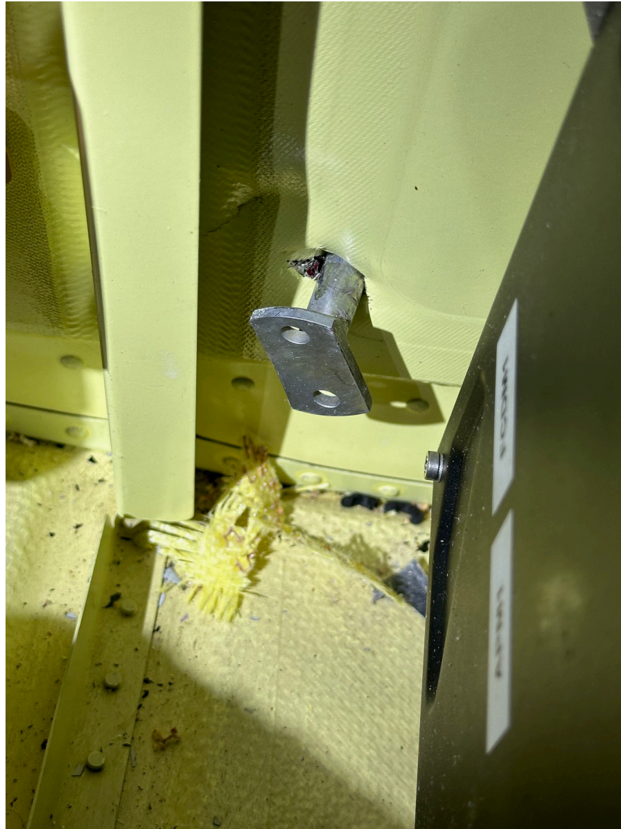
Photograph 4 - T-Bolt as found (Courtesy of Metro Aviation)
