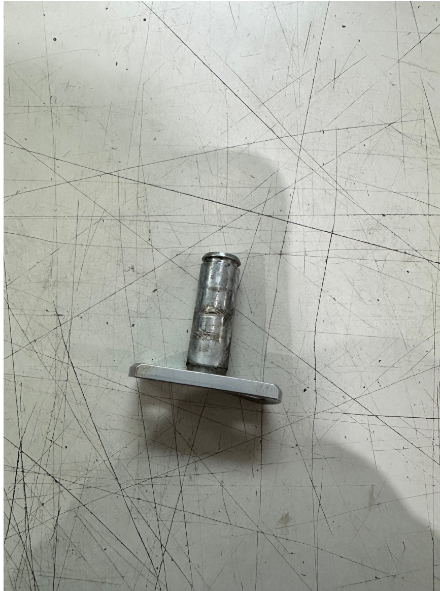
Photograph 7 - T-Bolt as found (Courtesy of Metro Aviation)
