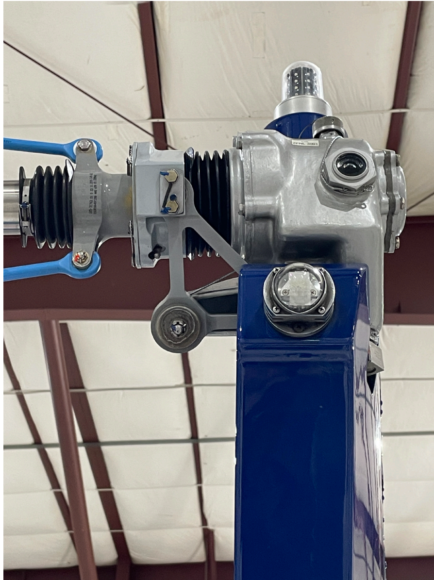
Photograph 3 - T-bolt installation on exemplar helicopter (Courtesy of NTSB)
