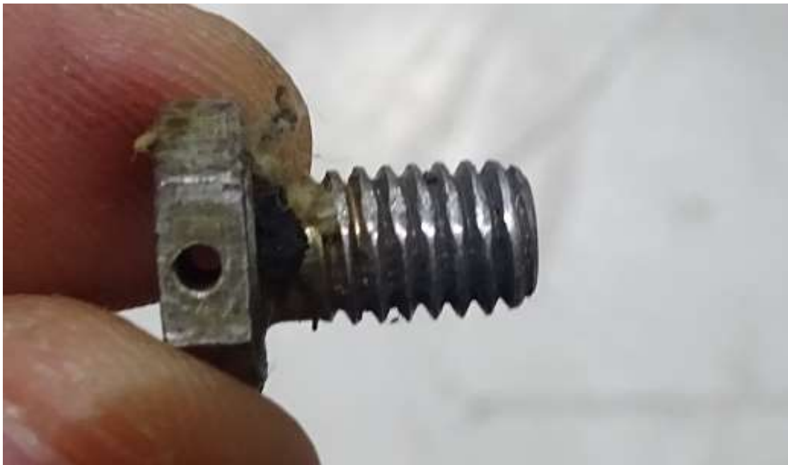
Figure 9. The second T-bolt attachment bolt, found near the No. 1 engine exhaust duct, exhibiting a flattened appearance on a portion of its threads.
