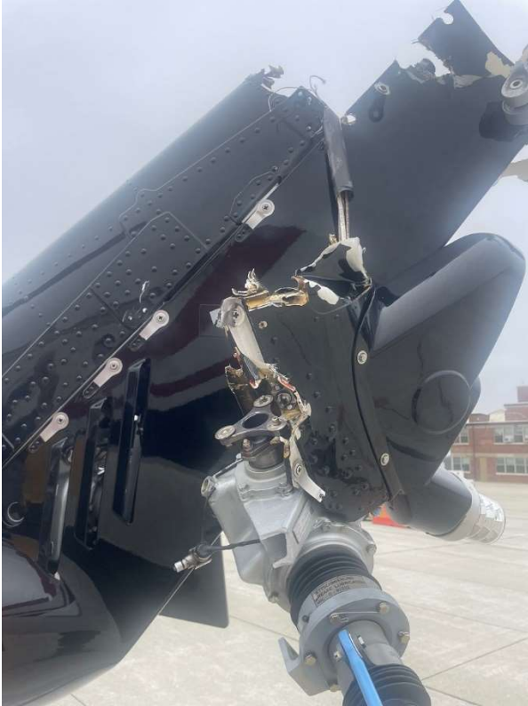
Figure 3. The tail gearbox attached to the separated upper portion of the vertical fin. (Courtesy of Metro Aviation)
