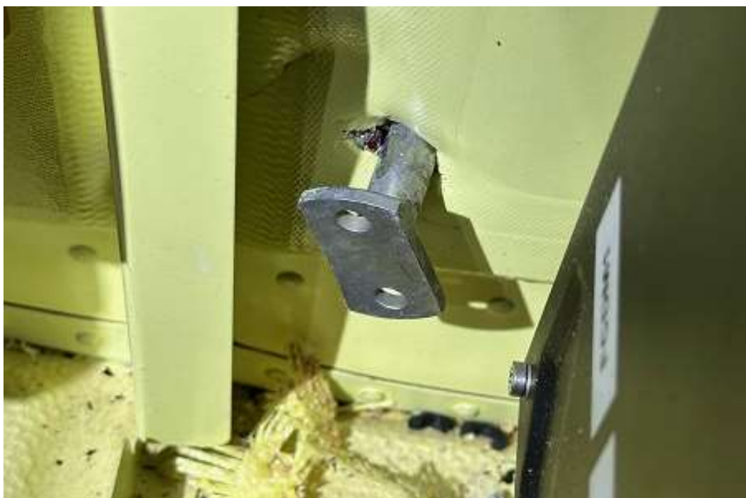
Figure 10. The T-bolt found lodged into a honeycomb panel. (Courtesy of Metro Aviation)
