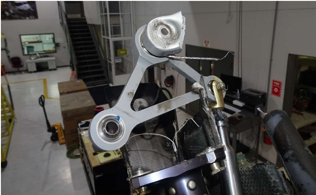
Figure 7. The pitch change bellcrank on the upper side of the vertical fin.
