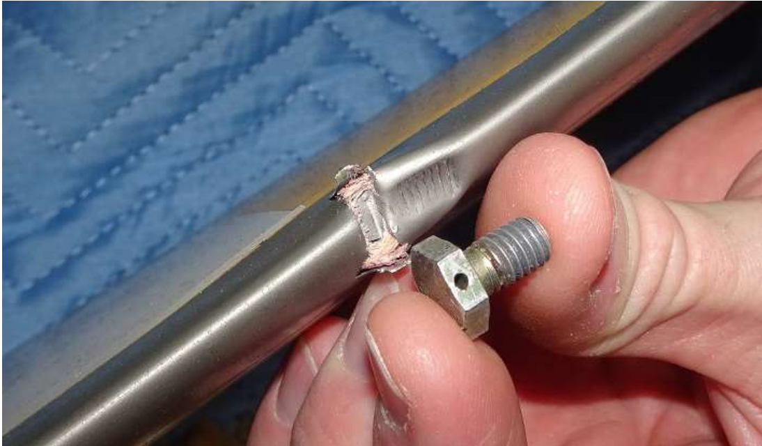
Figure 6. A T-bolt attachment bolt (found on the ground at the accident site) and the impact damage to the leading edge of tail rotor blade S/N 1511.
