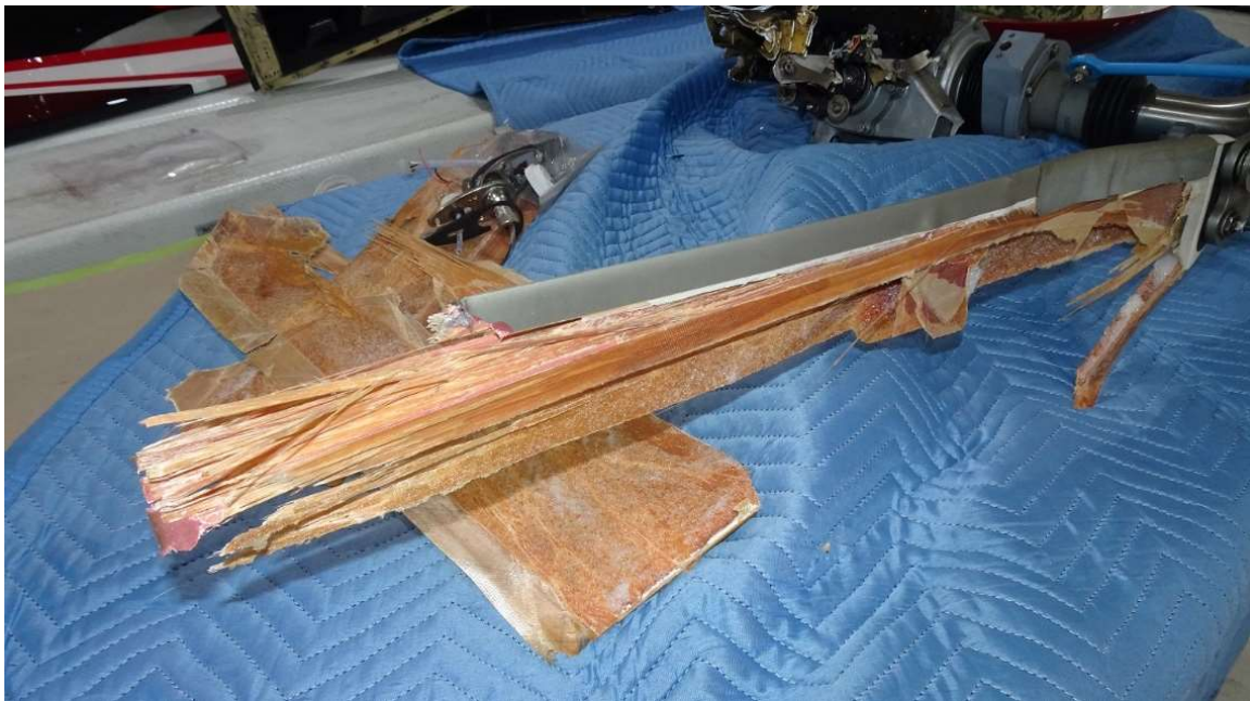
Figure 5. The tail rotor blade exhibiting a fractured leading edge abrasion strip and missing its afterbody.
