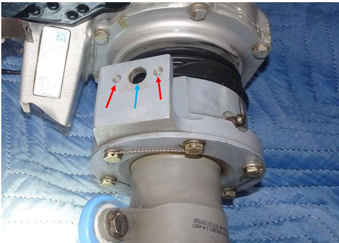
Figure 8. The pitch change slider with the holes for the T-bolt (blue arrow) and T-bolt attachment bolts (red arrows).
