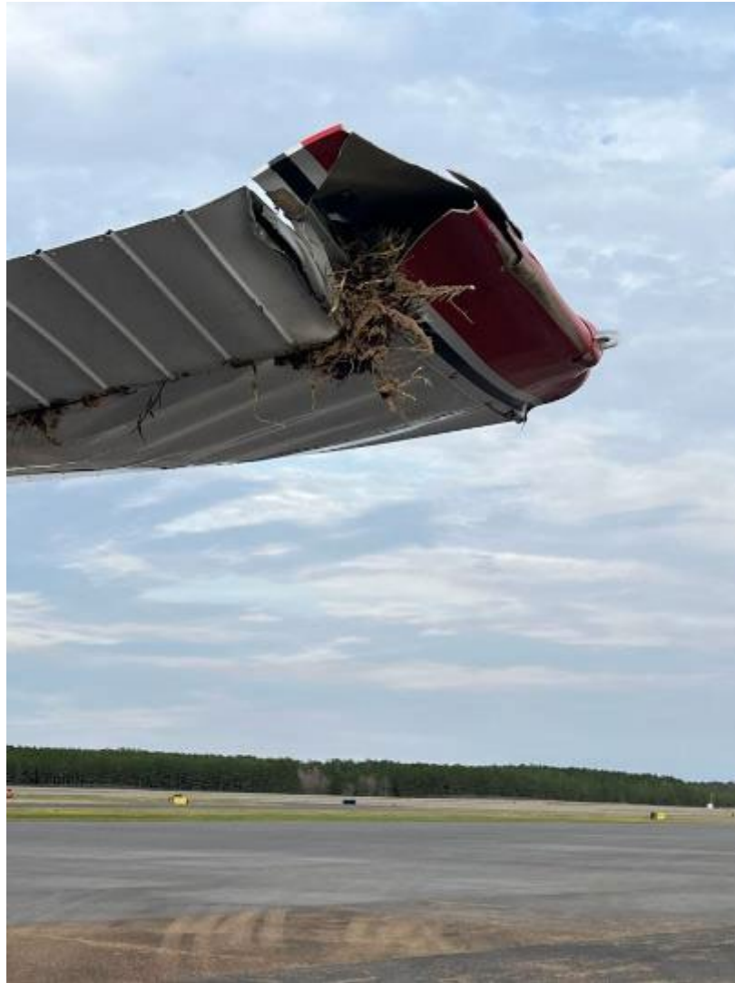
Photograph 3 - Accident airplane right wingtip (Courtesy of airport manager)
