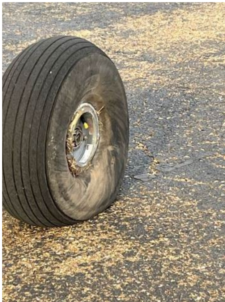
Photograph 4 - Accident airplane right wheel and tire assembly (Courtesy of airport manager)
