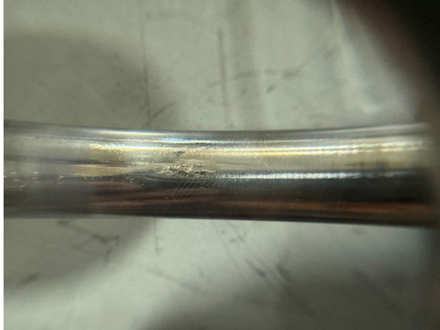
Figure 8. Metallic Like Debris on Exhaust Valve Stem
