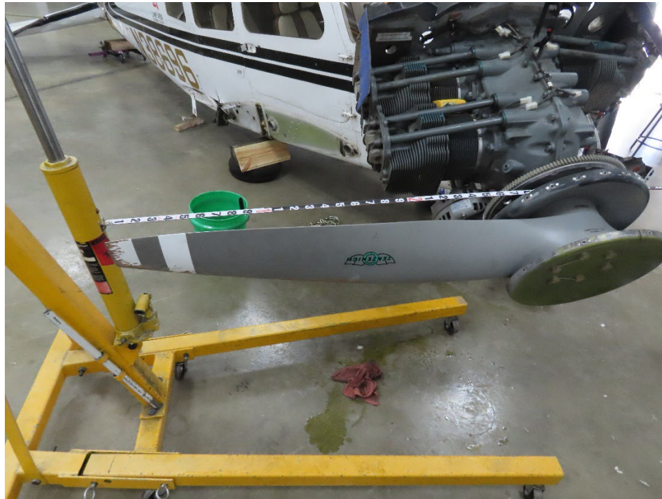
Figure 10. Propeller Blade A with Aft Bend.
