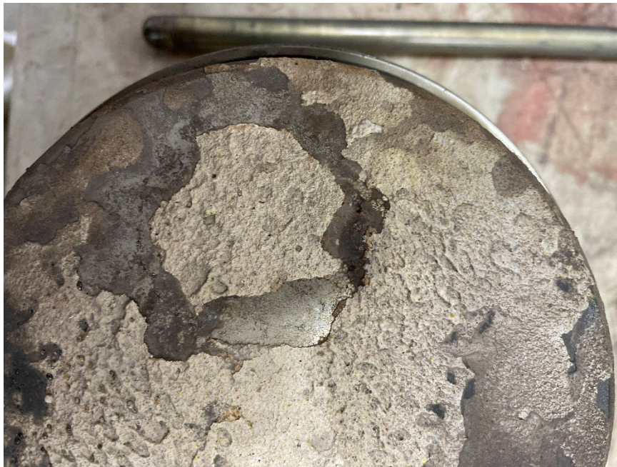
Figure 9. Circular Impression within Deposits on the Piston Head
