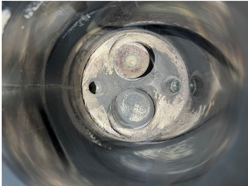
Figure 7. #2 Cylinder Inside View with Open Exhaust Valve (Upper)
